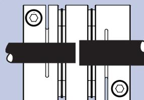
If the shafts of the equipment are smaller than the ID of the flex element they may be extended into the interior of the coupling. The ends of the shafts must never touch each other.
