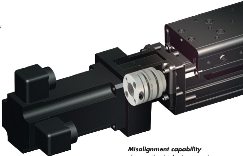
**Zero Backlash** is another key requirement of a high performance servo coupling. A coupling may be considered zero backlash and still have a large amount of torsional windup. Zero backlash and high torsional stiffness allow the coupling to maintain the same angular relationship between the input and output shaft without lost motion. The Zero-Max ServoClass coupling is a zero backlash coupling and it exhibits a very low amount of windup.
