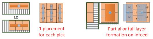
With the integration of a smart conveyor, the palletizing production rate can be significantly increased. A smart conveyor can bump turn the boxes before a pickup. This will eliminate the need for individual box placements when the build requires a row of rotated boxes. Some smart conveyors can create a partial or complete layer formation at the infeed. The powerful tools of the pattern generator will support both of these types of smart conveyor designs.
