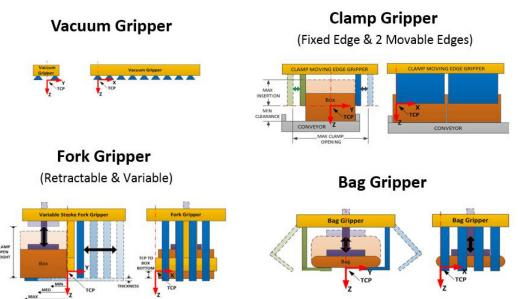
A gripper can be configured to have up to 32 grip areas. Each grip area is controlled by a set of I/O to grip, release and blowoff. These grip areas can be grouped into zones (maximum of eight). A key benefit is that the gripper can dynamically change its zone configurations for each infeed, depending on what size of box needs to be picked up. Refer to the following example:
