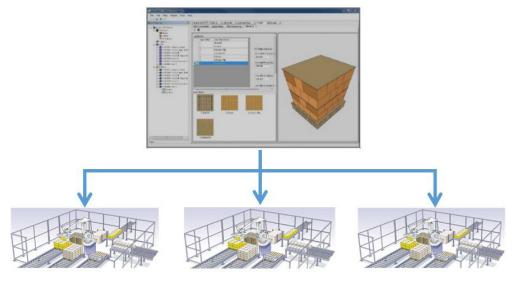
During production, when it is time to switch the pattern file for a particular line, an operator simply selects the file identified by the Product ID and Pattern ID, and downloads it to the robot controller. While the cell is executing, status is provided for all build stations, and errors are reported to the programming pendant (DX-series) or made available to the customized operator interface provided with the turnkey system (DX and MLX).
