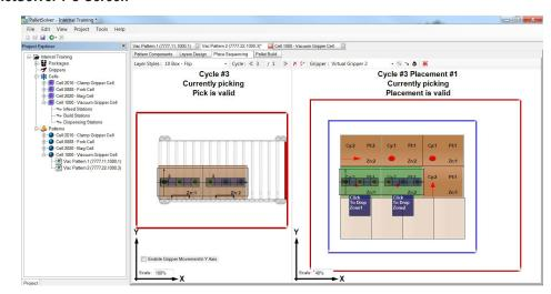
PalletSolver-PC software provides a key benefit of quick changeovers without halting production for validating pattern files. This is achieved by incorporating physical cell constraints of the workcell - such as distance between pallets or infeed stations, and interferences with neighboring objects or other build stations. Thus, the sequence for each pattern file is optimized based on constraints associated with that particular station ensuring the maximum production rate for each work cell.
