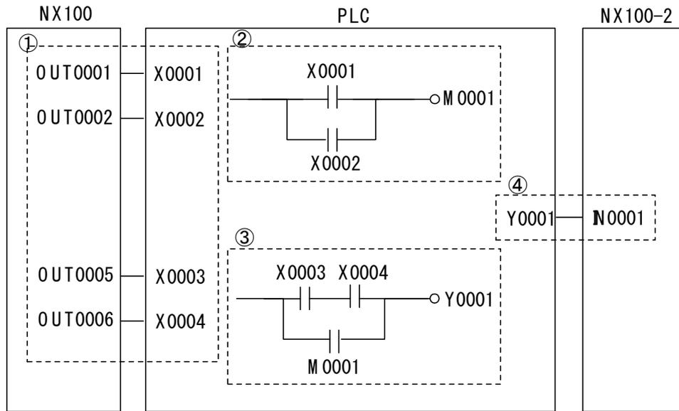
1. Set to substitute OUT001 of NX100 for X001 of PLC device.
