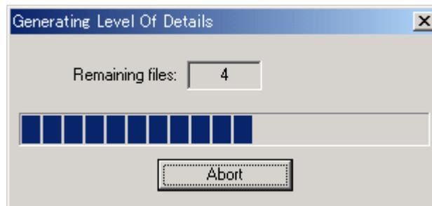
When adding HSF model and the Level of Detail is enable, the level of detail data will automatically be generated for the new model. The "Generating Level of Detail" progress dialog will display but the process cannot be aborted.
