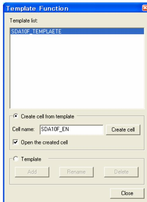
5. The new cell is created. If the [Open the created cell] is checked, the new cell is opened.
