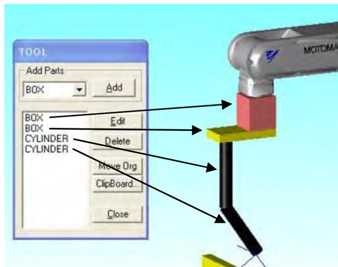
4. When the parts are all added, check the tool model on the screen, then click on the [Close] button to exit the file data editing dialog box.
