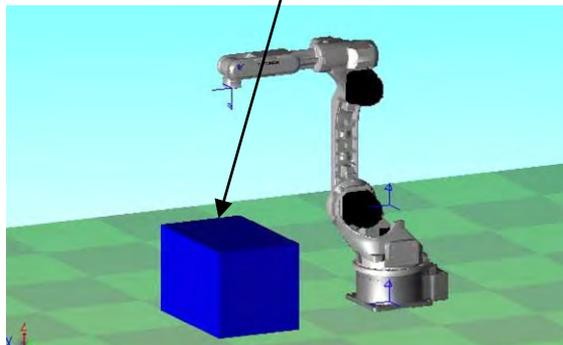
9. To create a workpiece, set "STAND" as the parent model by pointing the cursor to "STAND" in the Cad Tree. Create a new model named "WORK" as shown in the figures below.
