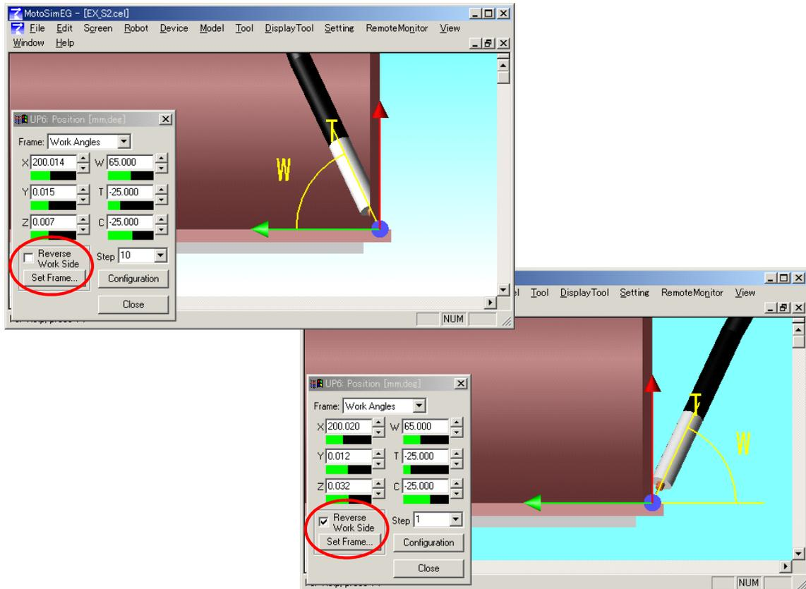
The Travel angle (T), also called the Push/Pull angle, is defined as the angle between the torch and the YZ plane. When set to 0 degree, the tool is in perpendicular to the travel direction. If "T" is positive, the tool is pushing; and if it is negative, the tool is pulling. The "C" angle is the rotation angle around the Tool Z axis.
