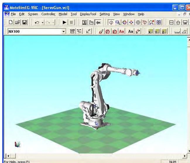
2. Display the CADTree dialog, then select the controller station (e.i. NX100-ST1). Move this model to the robot TCP model (e.i. NX100-RB1\_tcp) with the “Move Parent” function.
