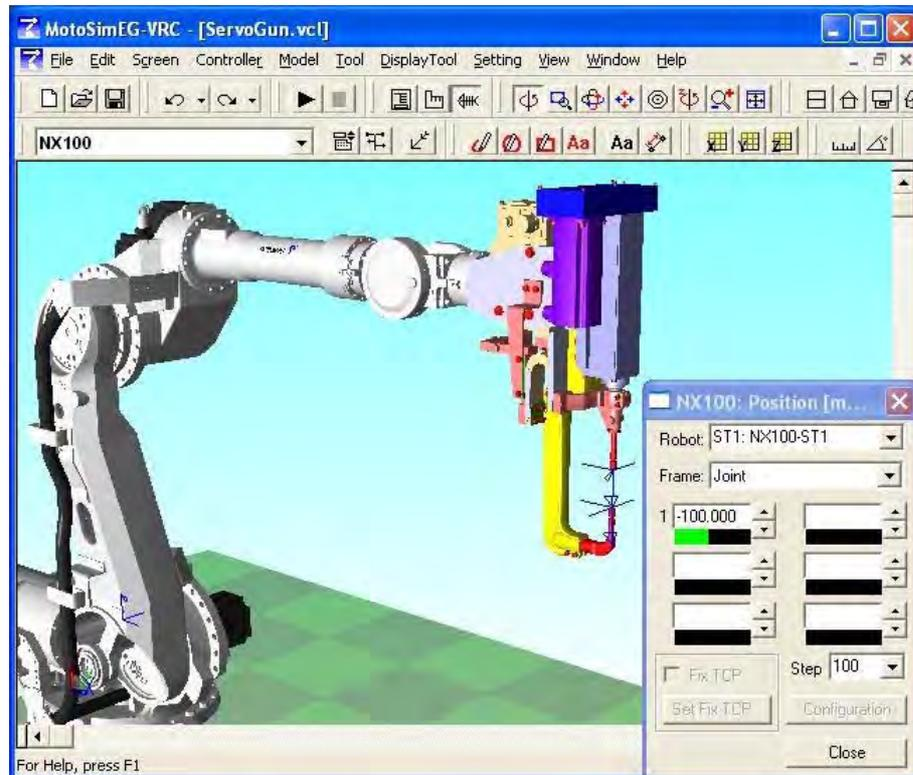
If the model doesn't move in the proper direction, you may need to adjust the orientation of the station axis 1 location frame (e.i. NX100-ST1\_EX1-POS) and then readjust the Motor Gun mobile part model.
