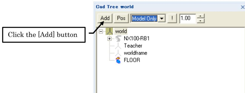
**NOTE** To create a new model in the model selection screen, verify that the cursor is pointed to "world" so that it will be the parent model.
