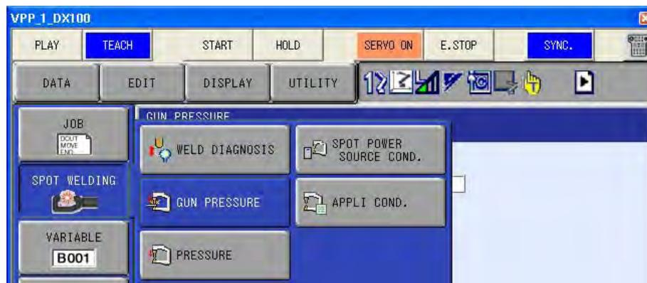
3. The setting of the gun pressurizing power is changed.
