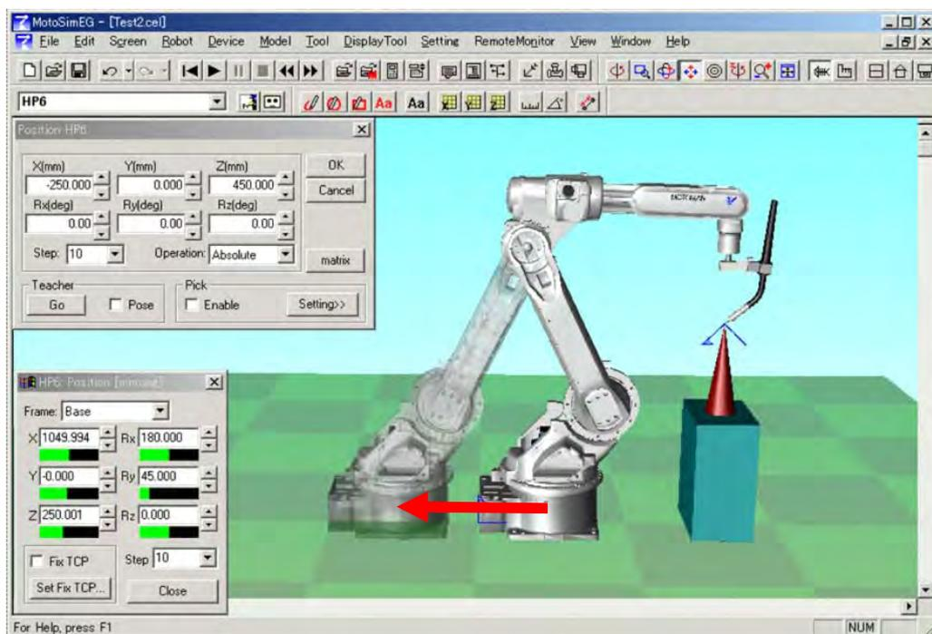
It can also be used when teaching a robot with an external axis. After the tool has been set in position, if the robot external axis needs to be changed, with the Fix TCP function enabled, the robot tool will remain in position. This avoids having to adjust the robot tool after moving the external axis.
