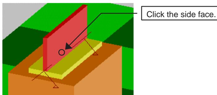
3. The tool end moves to the center point of the designated model face or edge. If the tool overlaps on the model, the tool direction is improper. Use the programming pendant to correct the position afterward. Click on another face to check if the tool end moves to the center of the designated
