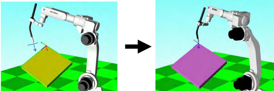
If the [Orientation] checkbox is not checked, the direction of the tool coordinate axis will not be changed as shown below.
