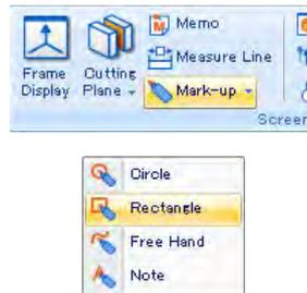
Position the mouse pointer at a desired point, and drag the mouse: a rectangle is drawn from the point where the mouse started dragging.
