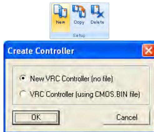
2. The "New Controller" dialog box appears. Select the controller type and then the system version from the list below. If desired you may change the default name for the controller. Click the "OK" button.
