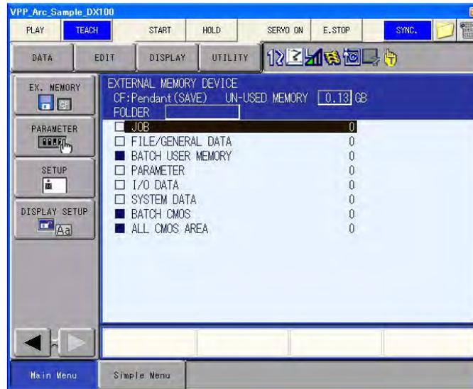
2. Select the type of data to be saved. For the figure below, {JOB} was selected. The list of files (in this case, the list of jobs) will display.
