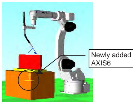
The AXIS6 is inside the BOX. (To see AXIS6 make sure that the Axis6 are always displayed in front in the "Options" dialog. Please refer to Section "10.1.5 Frame & AXIS6")
