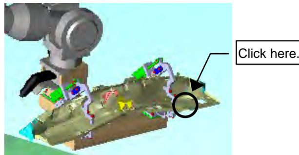
6. The robot will move the work piece target point to the external reference point.
