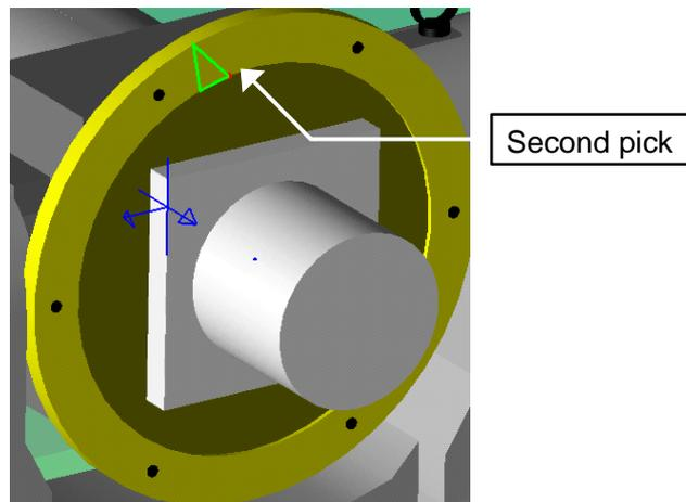
3. The point specified as the first point moves to the position of the second point.
