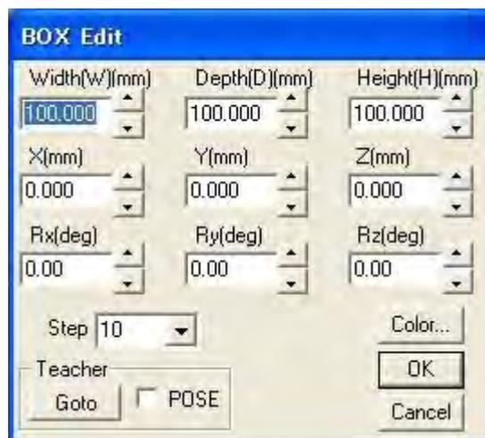
11. Set the workpiece size and position as shown in the table below in the BOX Edit dialog box: this model will be the bottom part of the fillet-welding workpiece.
