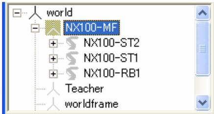
The dummy model "(Controller Name)-MF" is created. Robot model and MOTOFEEDER model are registered under the dummy model.
