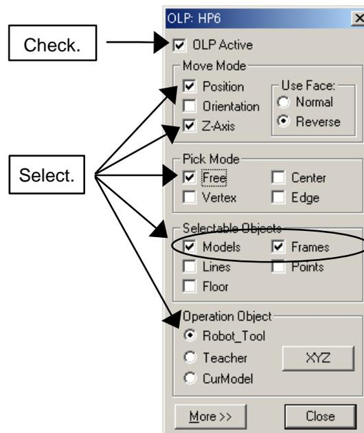
3. Click on the face of the "Work2", and the tool Z-axis will turn so that the tool end is per-
