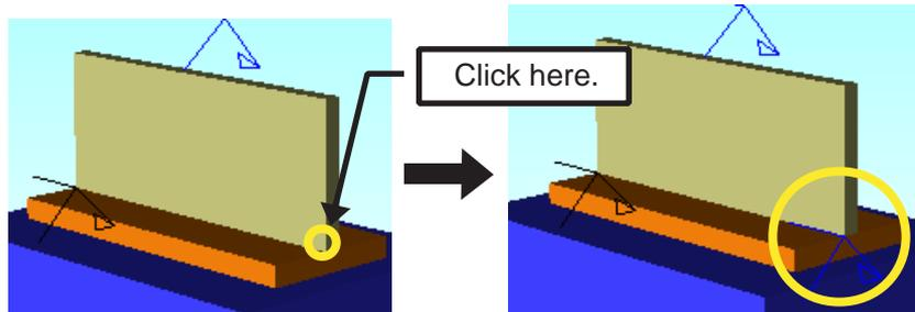
7. Add frame number 2 by clicking the [Insert] button in Frame Edit dialog box for AXIS6 which has been previously set; verify that the [Pose] check box is checked and click on [Goto].
