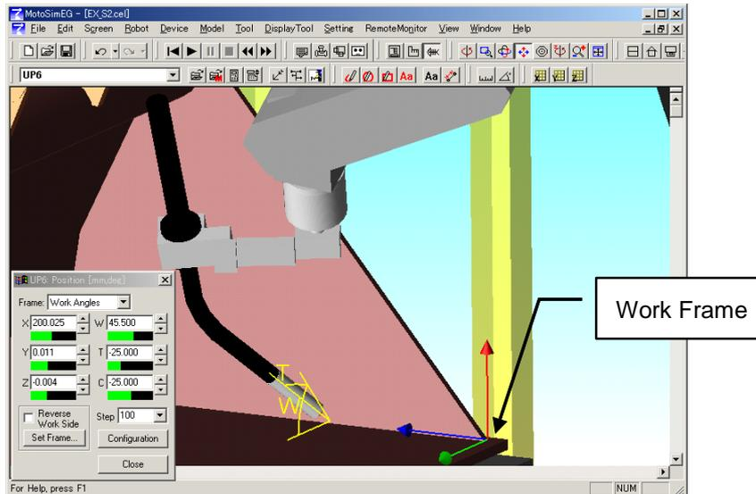
The Work frame is defined by three components: the frame position (or origin), the travel direction, and the work surface. The normal of the work surface is set as the Z-axis (red arrow) and the tool travel direction is set as the X-axis (blue arrow). The Y-axis (green arrow) will be set perpendicular to the other two axes.
