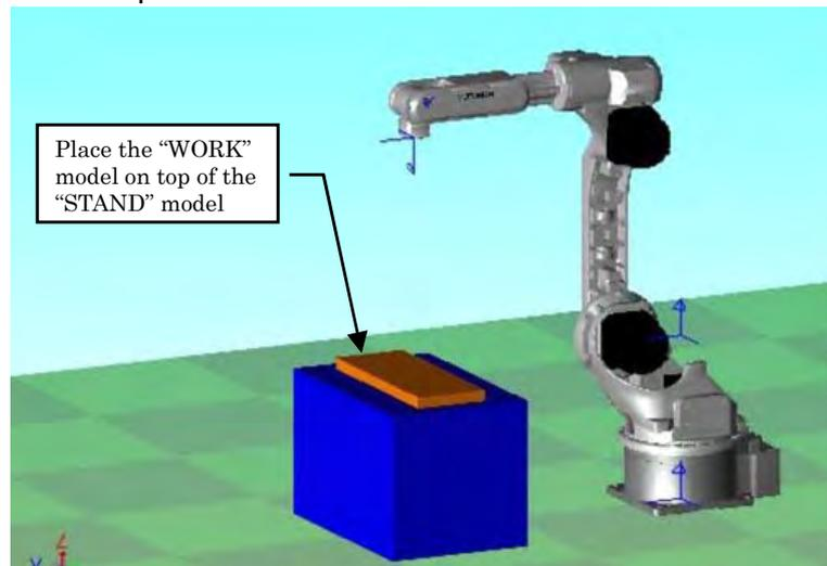
13. Create the upper part of the workpiece: the upper workpiece is composed of a second BOX part. Double-click "WORK" in Cad Tree to call up the file data editing dialog box, and add another BOX model (note that this operation should not be done by clicking the [Add] button in the Cad Tree).
