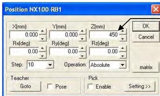
Distance between the robot frame and the floor.
