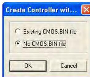
6. Select the controller system version, then press the [OK] button.
