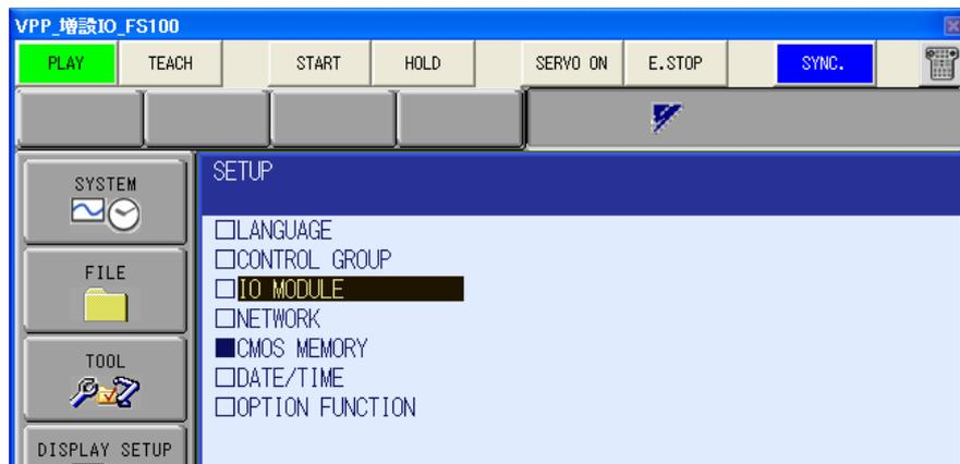
7. The list of [IO MODULE] is displayed. Confirm that the boards added in the "HwEmu.ini" file are present. After Confirming, click the [ENTER] button.
