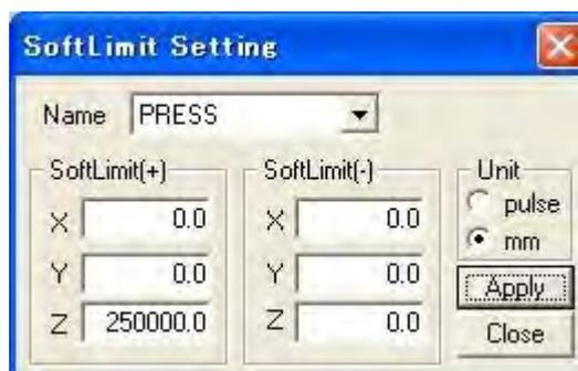
3. Modify the values as required and press the [Apply] button to make the modification.
