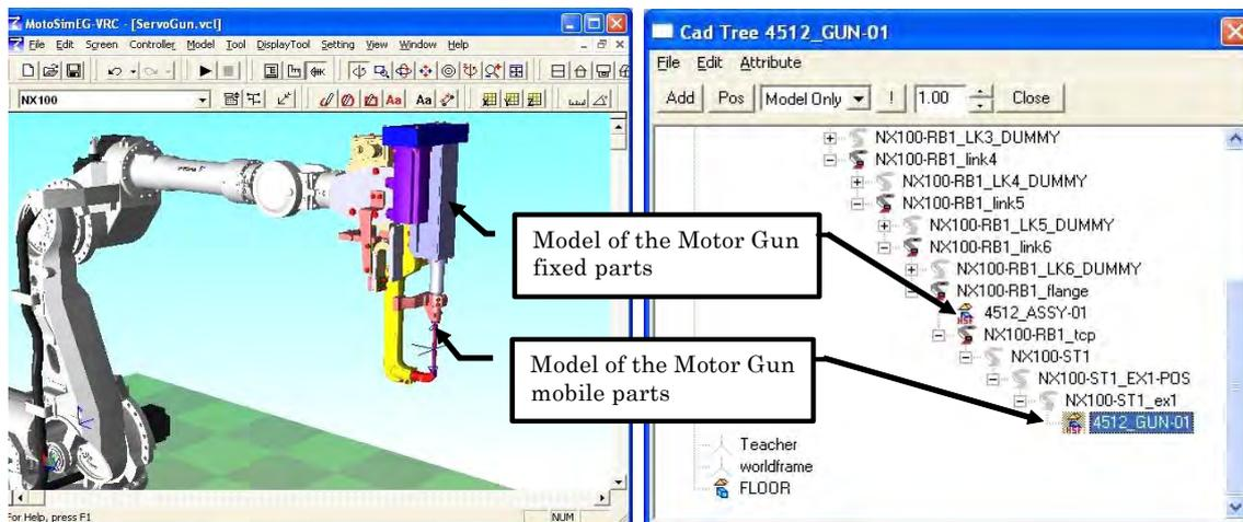
6. At this point, if the station axis is moved, the model will rotate around the Z-axis instead of moving along it. To change this, save and close the cell.
