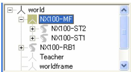
The dummy model "(Controller Name)-MF" is created. MOTOFEEDER model is registered under the dummy model. Robot model is registered under the world model.
