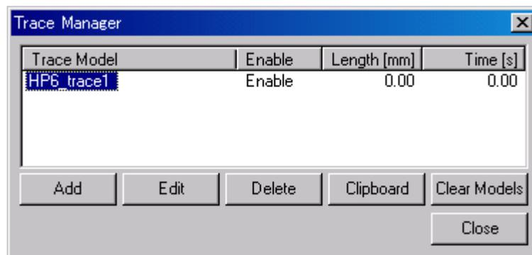
2. Display the trace property by double clicking on the “HP6\_trace1” or by pressing the “Edit” button. Press the [...] next to the “Model” field to display the “Select Model” dialog and select the model to be traced. For this example, select the “HP6\_flange” model. Then click on the [OK] button. Make sure that the “Model” edit box shows the selected model name and click on the [OK] button.
