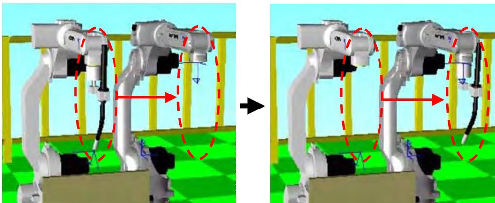
6. You can set the location of the VRC robot to overlap the MotoSim EG robot. (For details, refer to section Section "9.5 Positioning a Model".)
