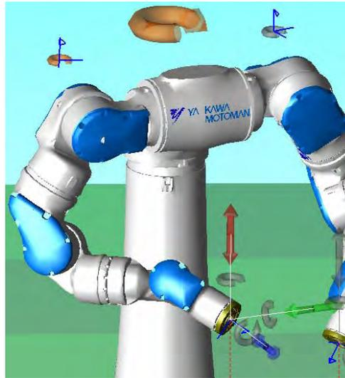
Tool axis: TCP handle always moves with position and posture same as TCP.
