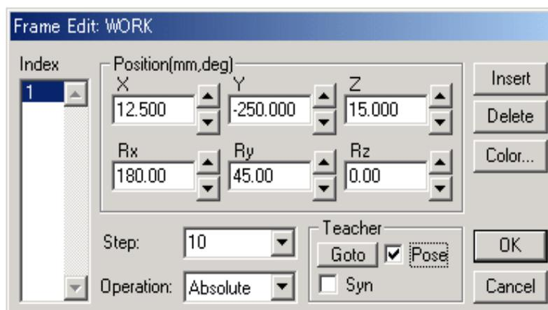
6. Set AXIS6 to the welding end point by performing steps 1 and 2 again, however, since the welding end point is to be set this time, be sure to click the part shown below in the OLP function. (Since the teacher angle has already been modified in the 3rd step, the angle modification is not necessary here.)
