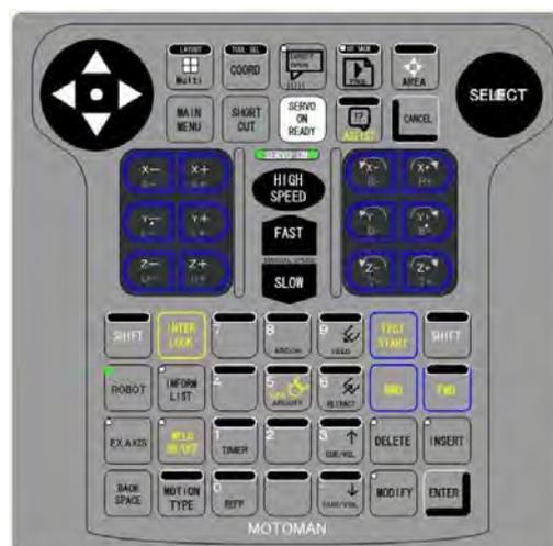
2. In the input line, select the motion type using the [MOTION TYPE] key of the pendant keypad.
