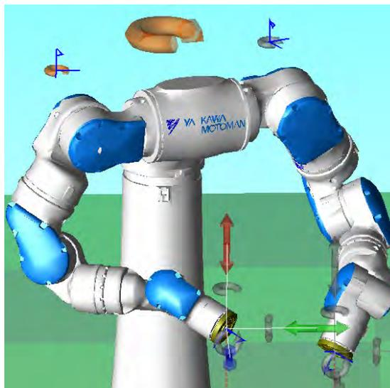
Robot axis: TCP handle always moves with posture same as a robot coordinate.
