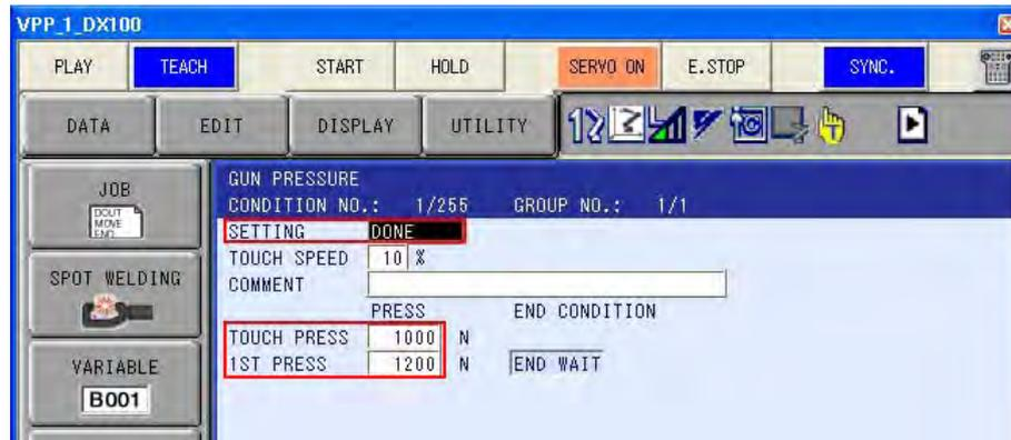
4. The main menu {SPOT WELDING} - {GUN CONDITION} of a virtual pendant is selected.
