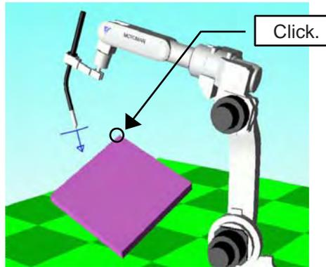
7. The tool end moves to the model vertex and the tool coordinate axis is aligned in the same direction as the target point frame that was displayed when the point was clicked.
