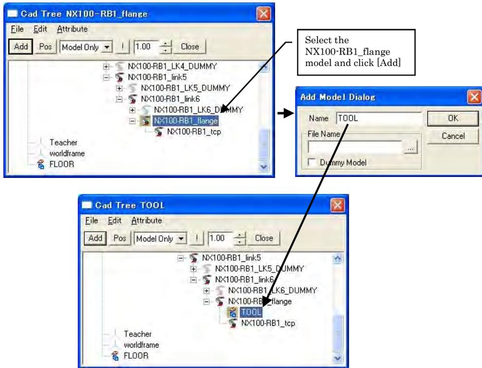
If the parent model is not set correctly, change the parent model by selecting {Model Attribute} - {Set Parent} as shown in the following figure.
