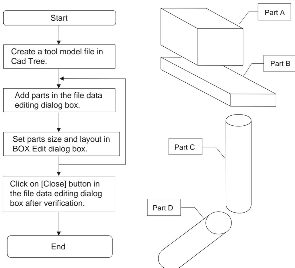
1. Display the Cad Tree to create a new model names "TOOL". In this case, point the cursor to "NX100-RB1\_flange" and create a new model so that the parent model of the tool model is the flange of the robot.
