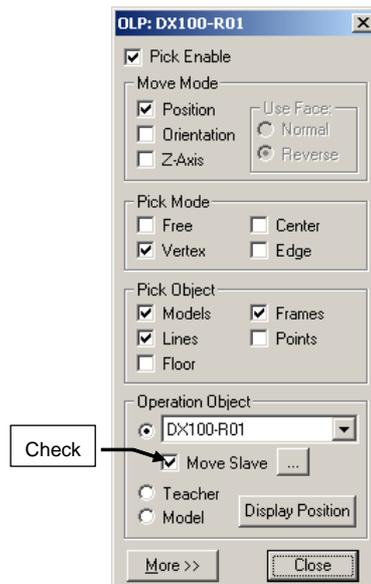
2. To display the "Set Slave Robots" dialog, click the [...] button. Then set which robot are slave robots.
