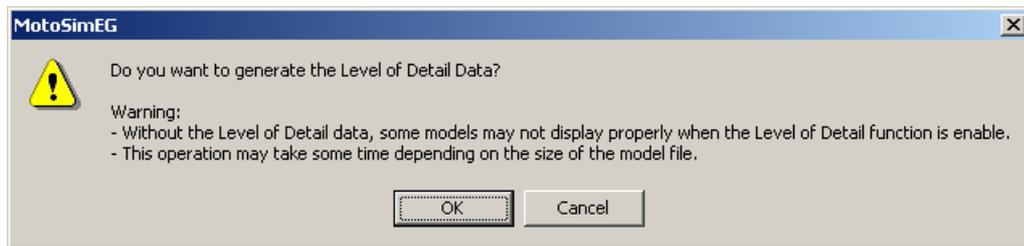
While generating the level of detail data, the "Generating Level of Detail" dialog will display the generation progress. To stop the data generation, click on the "Abort" button. Note that when aborting the generation, the current file processing will continue until completed, and then the generation will stop and data for the remaining file will not be created
