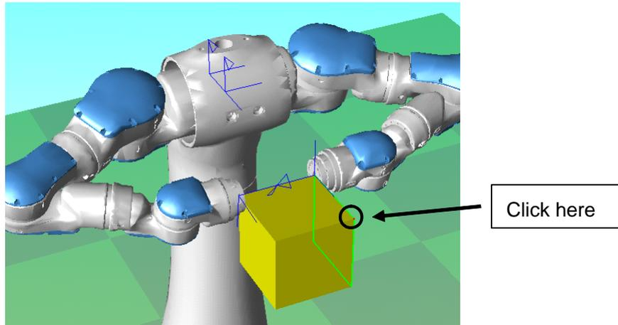
4. Then, slave robots are moved with it so that their TCP maintain the same relative position to the moved robot or station.
