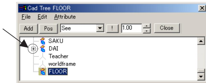
2. Select {Edit} - {Save Model Group} from the Cad Tree right-click menu. Select [Yes] to create a folder with the same name as the model selected in the step 1. The files of the model (selected in the step 1) and its child models are copied to the folder, and a parent-child relevant information file "ModellInfo.dat" is generated.
