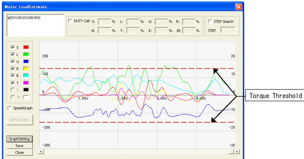
3. After the playback of a job, if the presumed torque exceeded the threshold value, the dialog will be displayed as follows.
