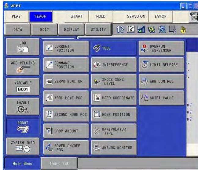
2. The TOOL settings appear. Move the cursor with the arrow keys to the Z field. Press the [Spacebar] to select the Z field for edition and enter the value "395". Press [Enter] to register the entered value. Repeat the same procedure for the Ry field and enter a value of -35. (In this example, the tool end curves by "Ry = -35" relative to the flange axis.
