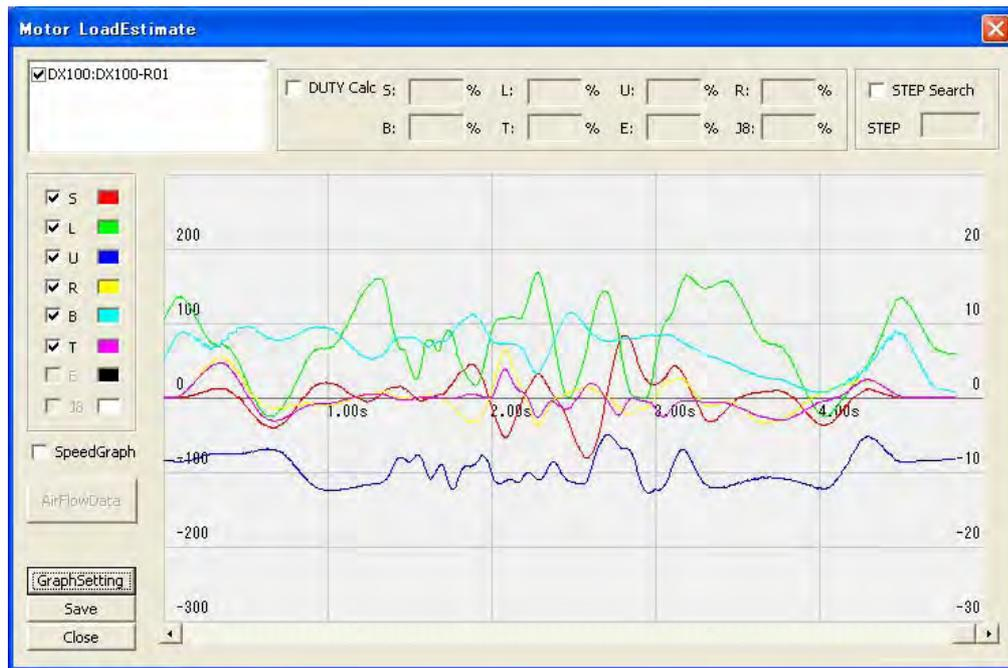
4. Select the axis that displays the torque estimate in the check box of the axis. (The axis can be selected even before the job is executed.)
