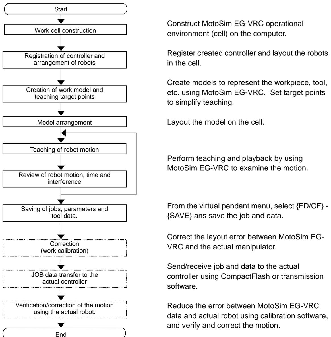
Solid lines indicate operation by MotoSim EG-VRC and dotted lines indicate operations by other software.
