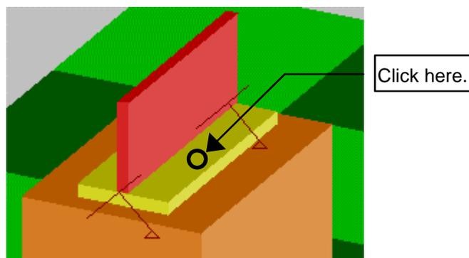
3. The tool end moves to the edge point nearest to the clicked position. Click on another face point to check if the tool end moves to the closest edge.
