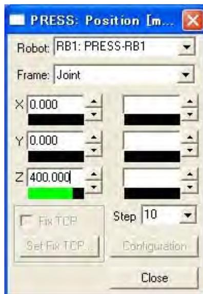
Gantry also have a station (external axes) mounted at the end of the robot TCP (X, Y, Z axes) that allows Rx, Ry and Rz rotations. To move this axis, change the selection in the robot
