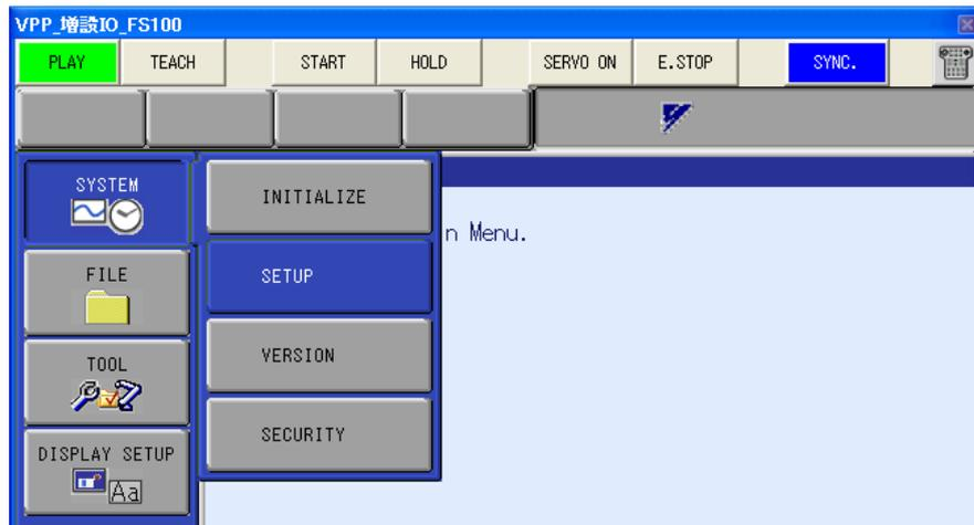
6. Select {IO Module} from the list in the {SETUP} display.
