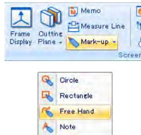
Position the mouse pointer at a desired point, and drag the mouse freely so that the mouse pointer on screen draws a line with the mouse movement.
