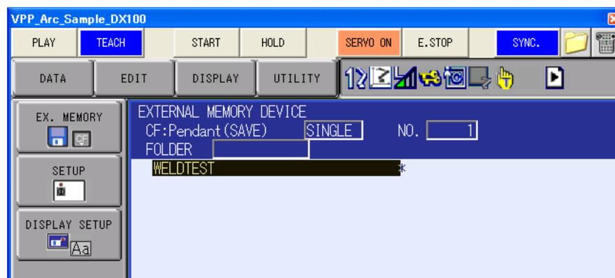
3. Select the files to be saved by moving the cursor on the file name and, press the [Spacebar] on the keyboard or click [Select] in the Virtual Pendant keypad. The selected files will be marked by a star ★ mark on there left.
