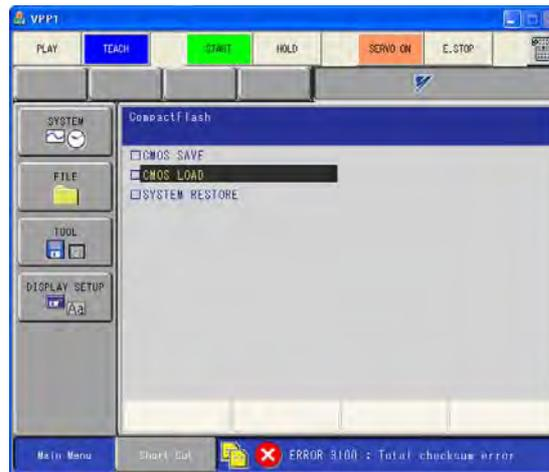
The CMOS cannot be loaded because the "VRC.BIN" version is from a controller version incompatible with the selected VRC version.
