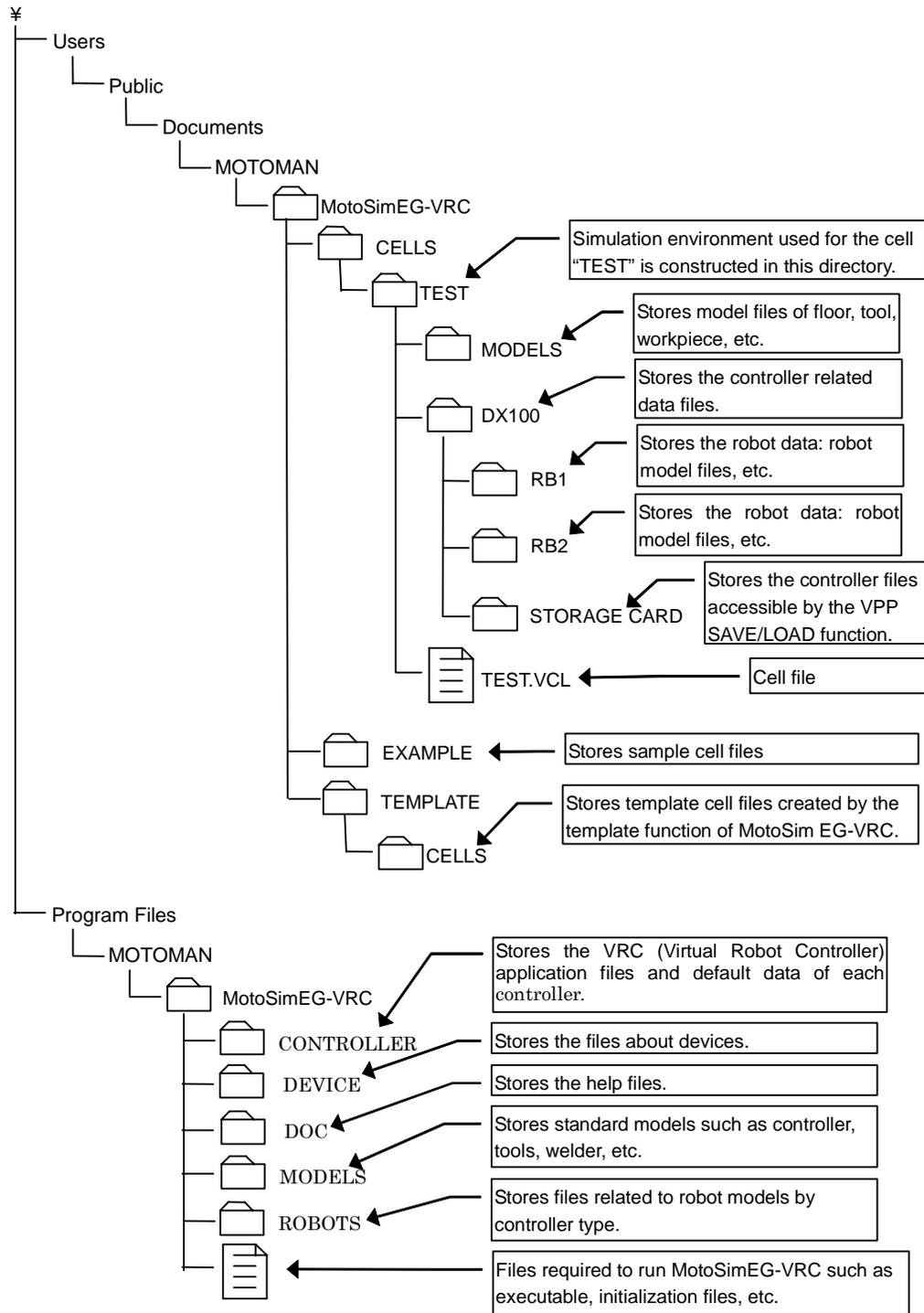
The above diagram is based on the assumption that the cell "TEST" is the file in which the simulation environmental data is stored, and that there is one controller named "NX100" with 2 robots defined under the folders "RB1" and "RB2".
