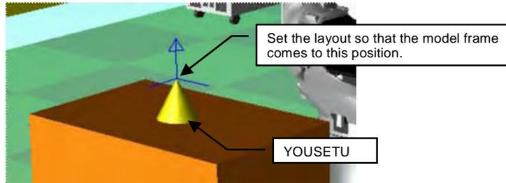
4. Create the “WORK3” model that has “TCP” as the parent. Select “HP6\_tcp” from the Cad Tree, then click on the [Add] button.
