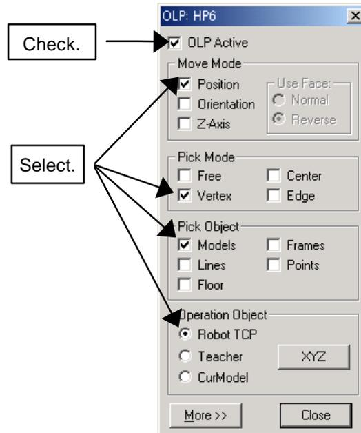
4. The tool does not move even though the "AXIS6" on the cell window is clicked. If you click around the vertex of the BOX, however, the tool moves to the vertex. This is because the [Frame] check box in the OLP dialog box has been cleared and only models are considered for selection.
