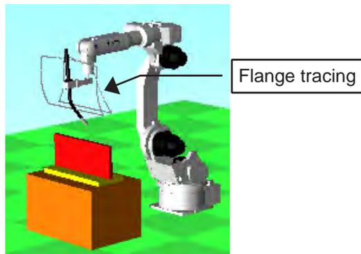
The following figure shows when the tracing point is a tool.
