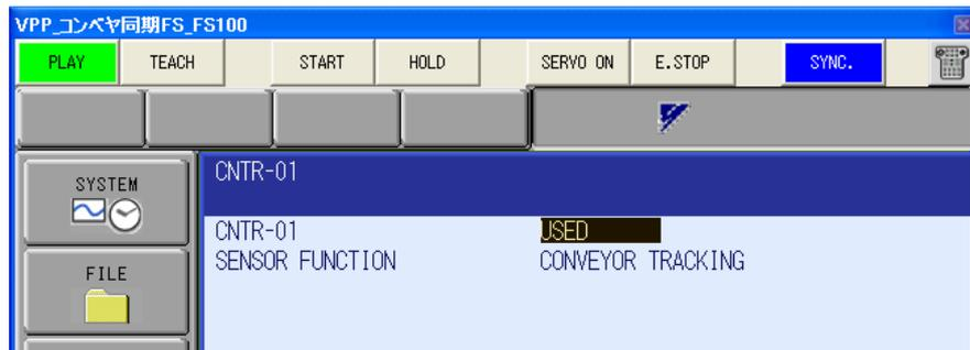
6. The "SENSOR FUNCTION ALLOCATION" screen doesn't need any change. Press [ENTER] to go to the next screen.
