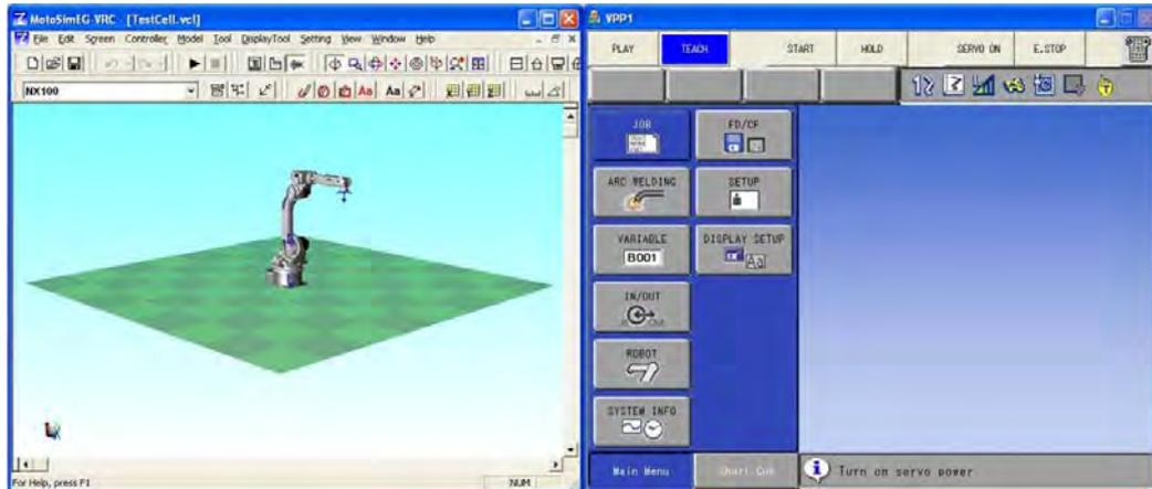
However, as shown in the following figure, the robot may be displayed as if it is sank in the floor. This is because the offset value of the robot operational origin and the floor center coordinate has been set to 0 (initial value). In this case, correct the robot position by following steps 10 and 11.
