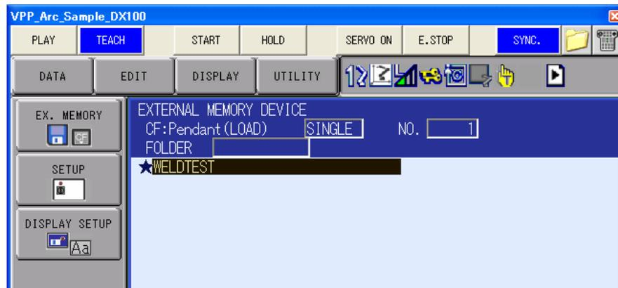
4. Press [Enter]. Select [Yes] in the confirmation dialog box that will display. The selected files will be loaded to the MotoSim EG-VRC controller.
