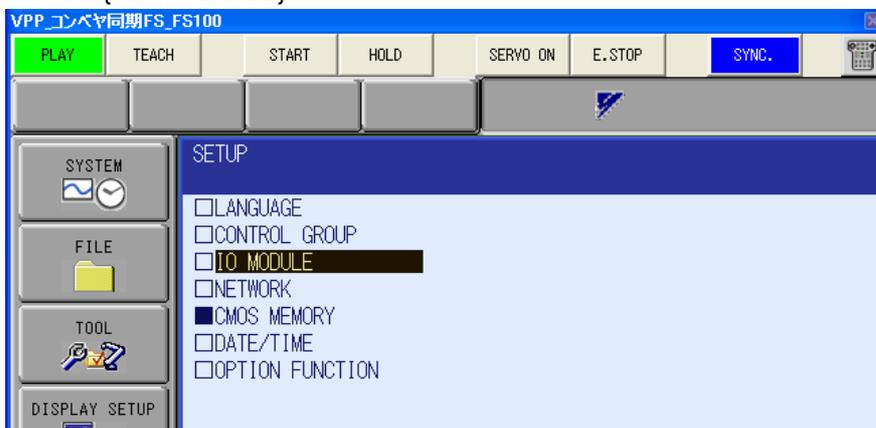
4. Select the [DETAIL] of the [CNTR-01] in the [IO MODULE] display.
