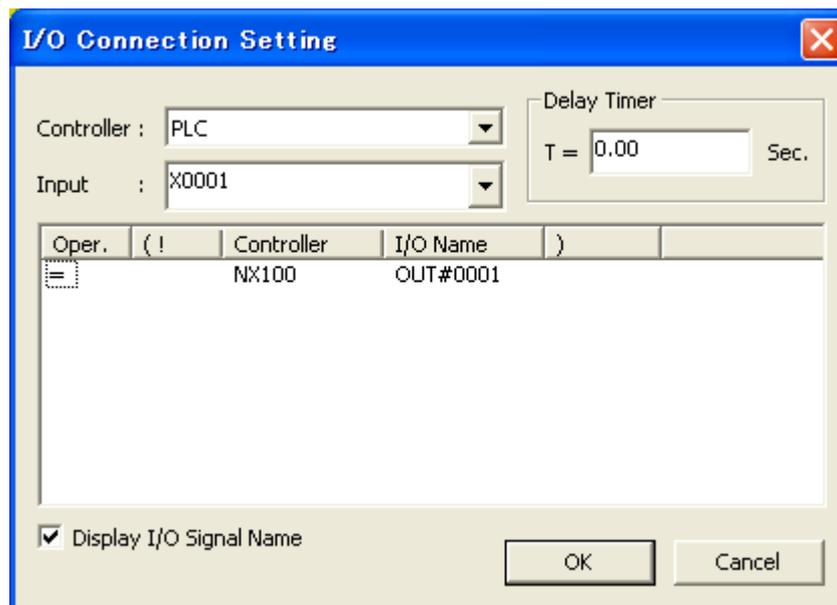
Also, "OUT0002", "OUT0005" and "OUT0006" set to substitute "X0002", "X0003" and "X0004" of PLC device.
