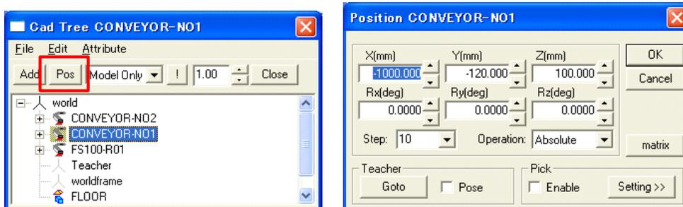
3. When the items other than the distance between the conveyors (Y direction) is changed, the following setting is needed.
