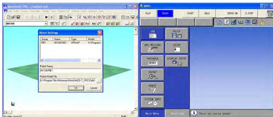
9. When the controller registration has been completed normally, the robot model appears in the cell screen as shown in the figure below.
