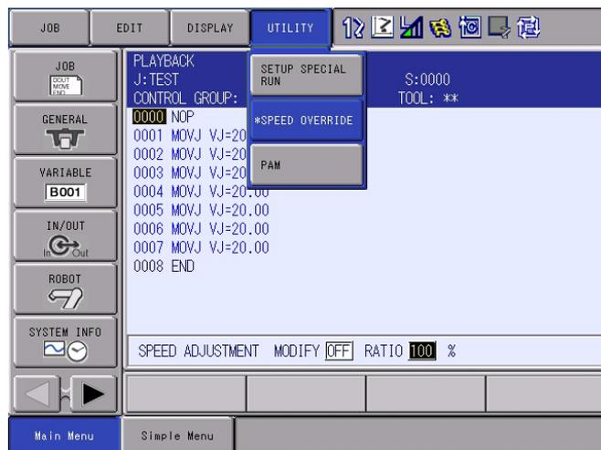
– When the speed override function is disabled, as shown below, the asterisk beside {SPEED OVERRIDE} and the "SPEED ADJUSTMENT" input buffer line disappears.
