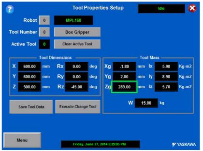
The Box Gripper TCP location needs to be the same as the gripper definition in the Offline pattern generator (PalletSolver -PC). Refer to *Fig.4-2 "Gripper TCP Examples"*.
