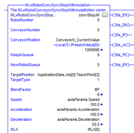
Fig. 6-16: Conveyor Synchronization Stop
