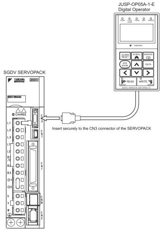
Note: JUSP-OP05A digital operators are used with Σ-III SERVOPACKs. A special connector (JZSP-CVS05-A3-E) is required to use these operators with  $\Sigma$ -V SERVOPACKs. For details, refer to Σ-V Series User's Manual, Setup, Rotational Motor (Manual No.: SIEP S800000 43).
