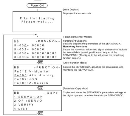
An abbreviation of the name of the active mode is displayed in the upper right, and the SERVOPACK status is displayed in the upper left.
