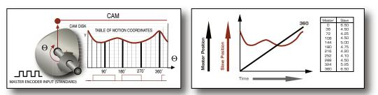
MotionWorks\* IEC includes 10 Function Blocks dedicated to camming. These are customized by Yaskawa based on the PLCopen specification, previous controller cam technology, and decades of synchronized motion experience. The function blocks fall into one of four functional topics:
