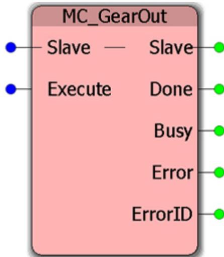
This Function Block disengages the Slave axis from the Master axis. The slave will continue to move at the last commanded velocity.
