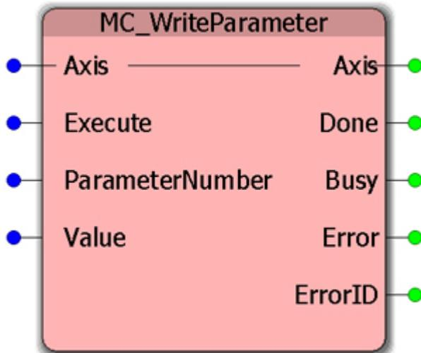
This Function Block writes the value of an axis-specific parameter and is for controller side parameters only. For amplifier side parameters, refer to [Y\\_WriteDriveParameter](#).
