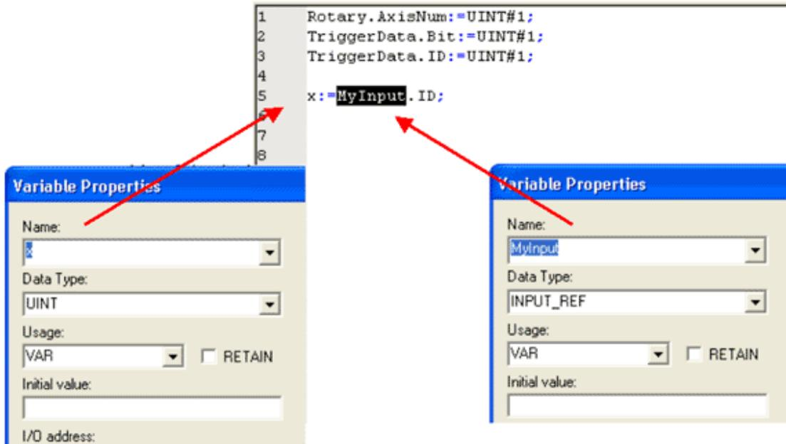
The image illustrates the configuration of variables in a PLC program. A code editor shows the following code:
