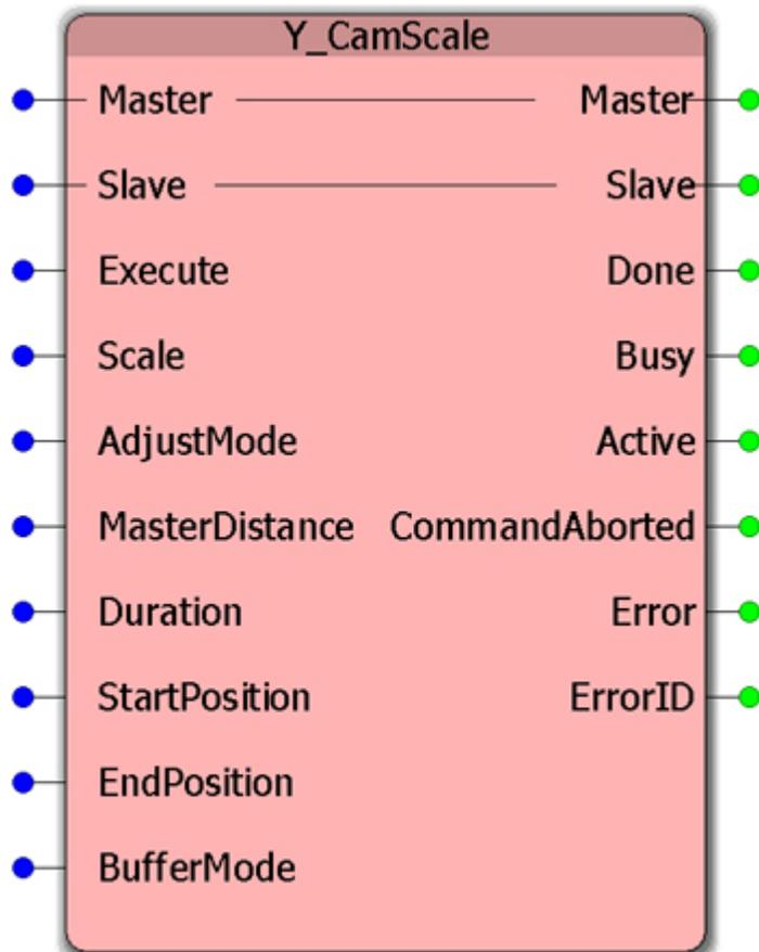
This Function Block multiplies cam slave position data derived from the cam table by a scale factor.
