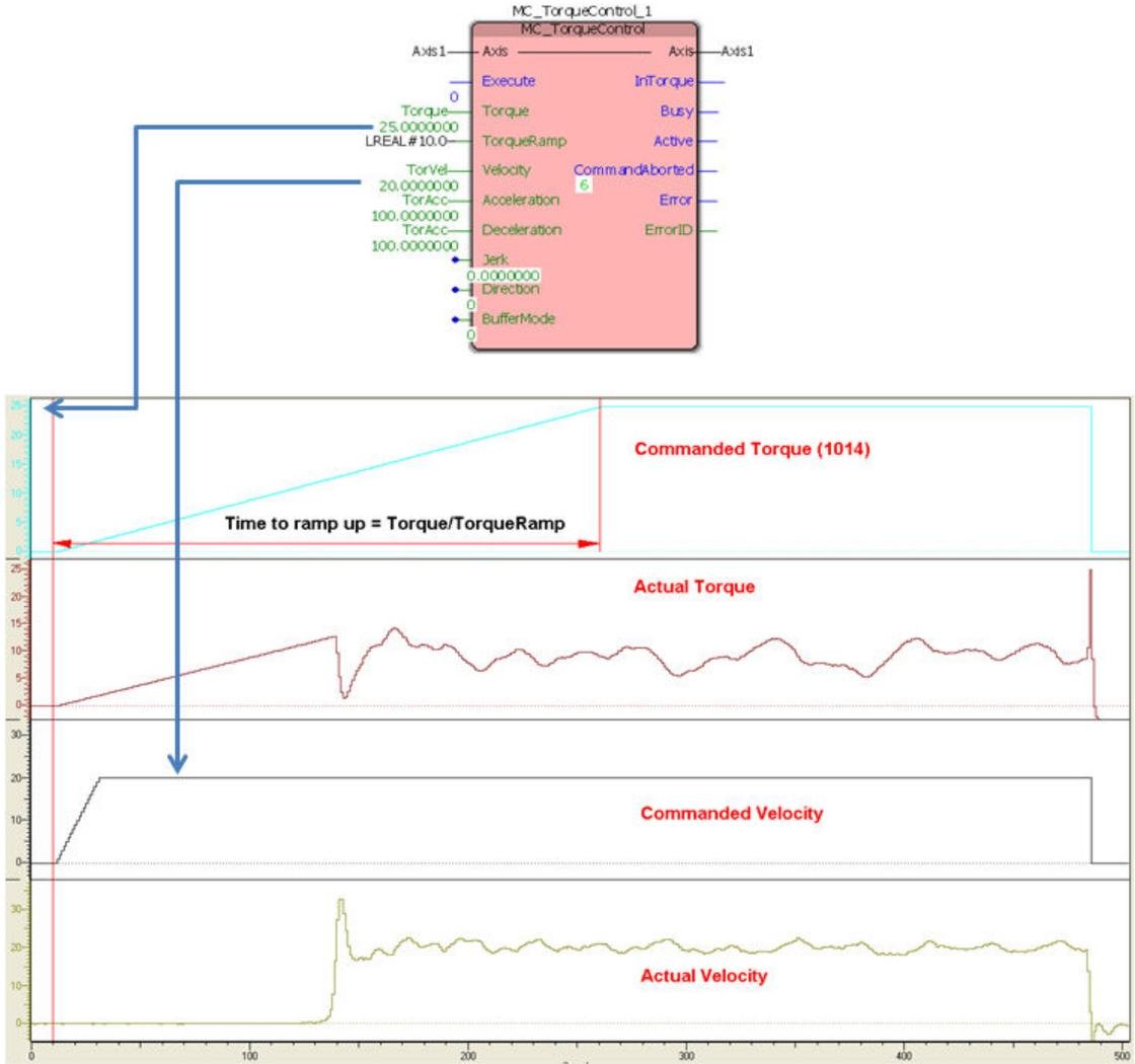
Sample torque and velocity profiles for an instance of MC\_TorqueControl
