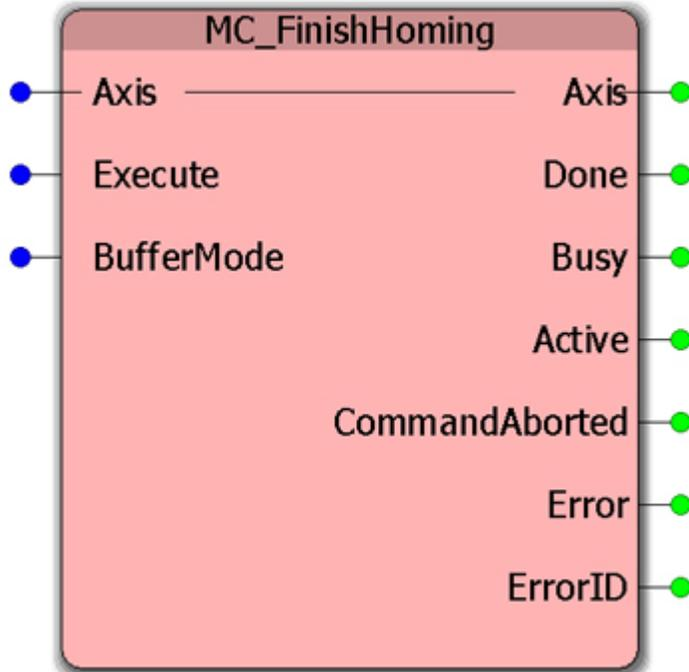
This FB transfers an axis from the 'Homing' state to the 'StandStill' state. It does not perform any movement. This block is necessary after the user builds a homing procedure containing any number of MC\_StepXXXX homing blocks (See Notes).
