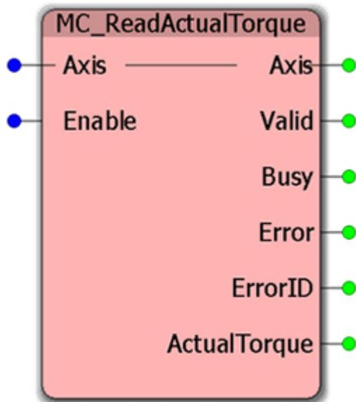
This Function Block returns the value of the actual torque or force in percentage of rated torque. Note that peak torque will vary from 200 to over 300% based on the specific amplifier model.
