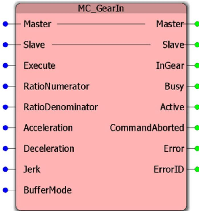
This Function Block commands a velocity ratio between the master and slave axes. If the gearing mode is executed while the master is already in motion, position synchronization will not be achieved unless some other method (MC\_MoveSuperimposed or MC\_GearInPos) is employed.
