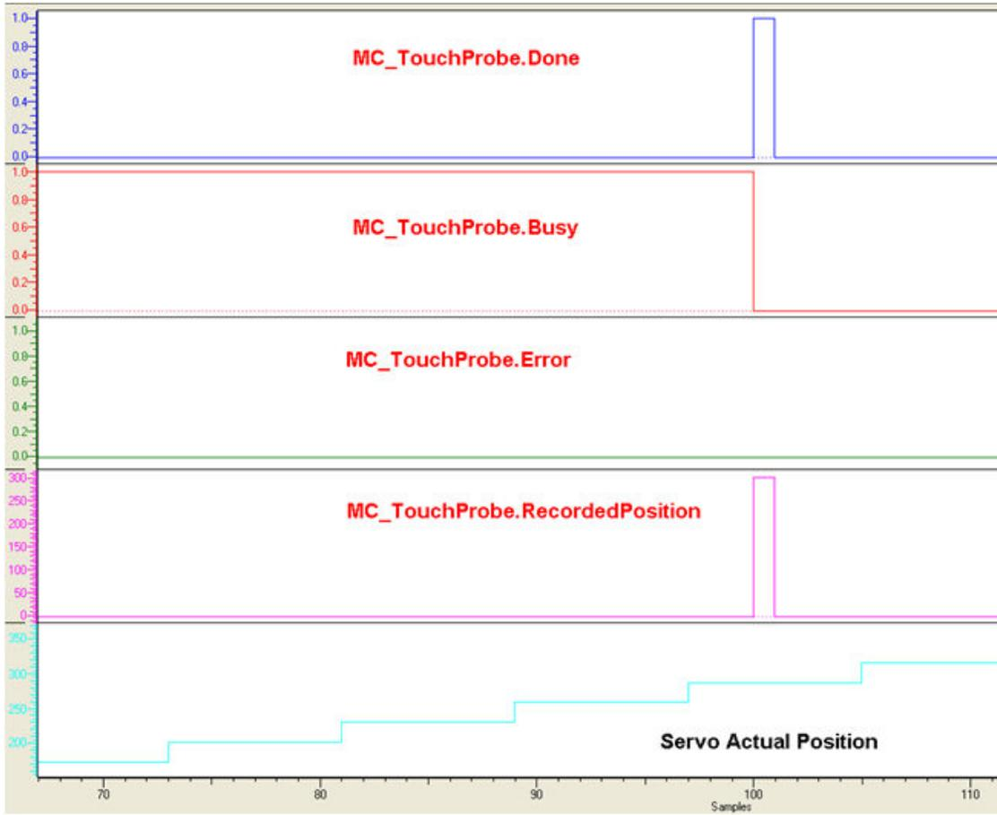
Timing Diagram for MC\_TouchProbe
