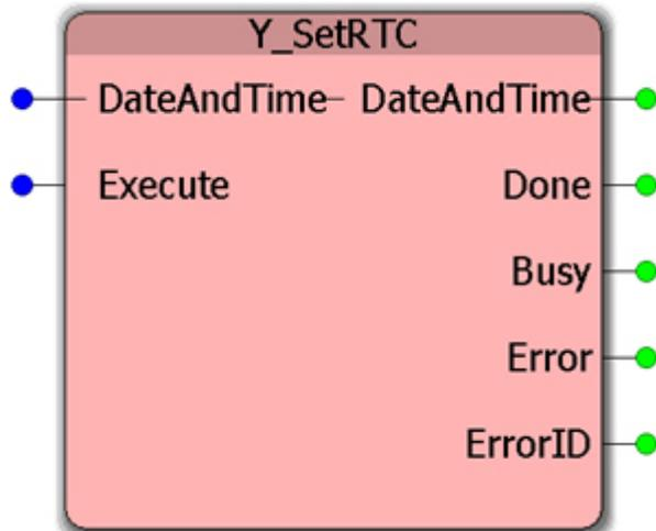
This Function Block allows the application program to set the controller's real time clock.
