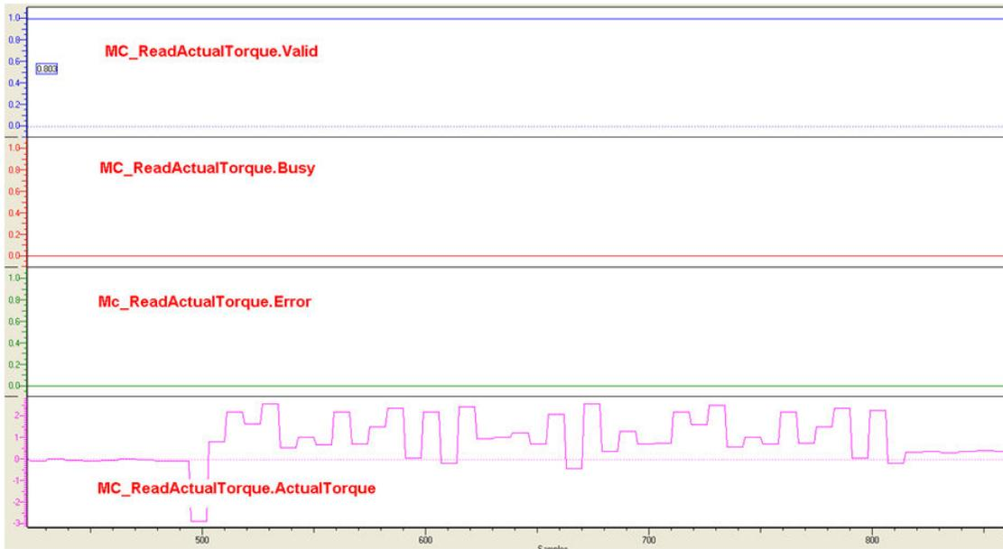
Timing Diagram for MC\_ReadActualTorque for a slow move of an axis
