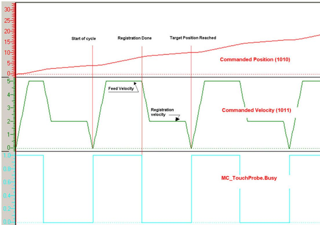
Timing Diagram for Feed to Length application
