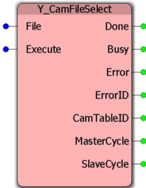
This function block loads a cam table from a CSV file into the motion memory.
