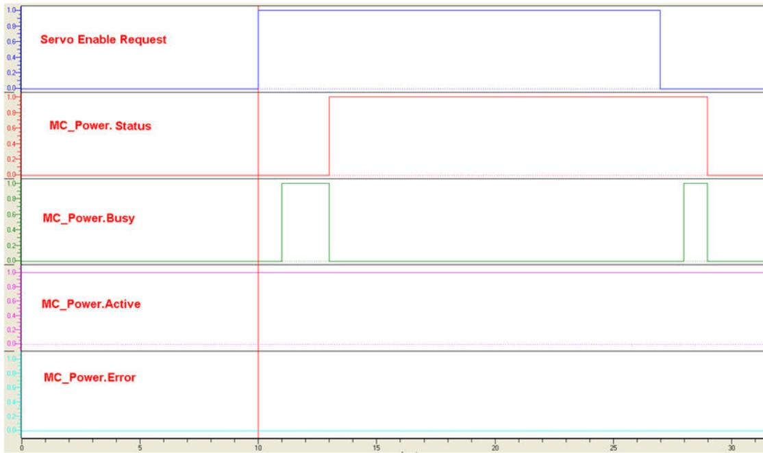
Timing diagram for MC\_Power
