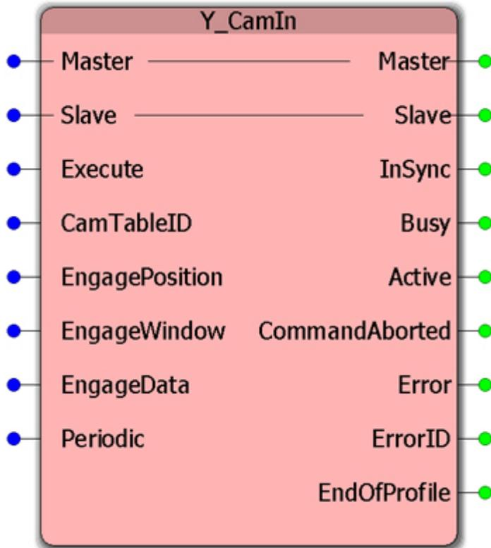
This Function Block engages the axis in camming mode with the cam profile specified by CamTableID.
