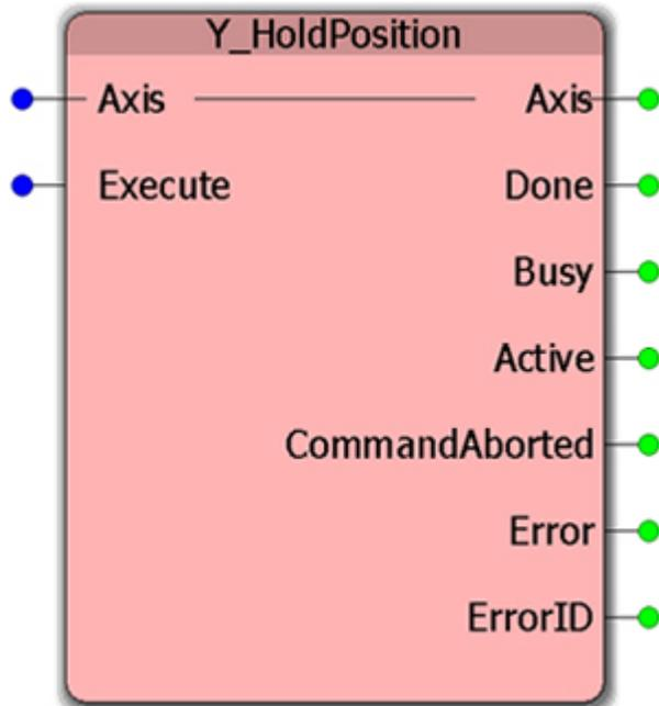
This Function Block commands an immediate position hold with maximum deceleration and changes the axis state to 'Stopping'. It aborts any ongoing FB execution. After the axis has held position, the Done output is set to TRUE immediately. As soon as 'Done' is SET, the axis goes to state 'StandStill'.
