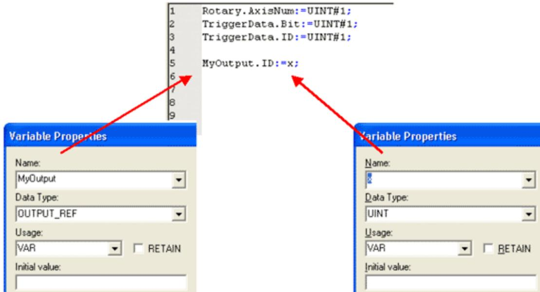
The diagram illustrates the configuration of the variable `MyOutput` in the code example. Two **Variable Properties** dialog boxes are shown, each pointing to the line `MyOutput.ID:=x;` in the code editor.
