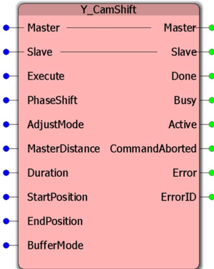
This Function Block dynamically modifies the master - slave relationship by adding a perceived offset to the master position, effectively causing the slave to advance or retard from the originally specified synchronization data in the cam data table.
