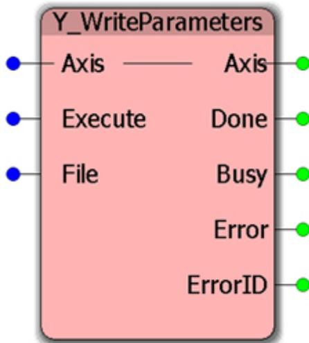
This Function Block writes all parameters to the drive as stored in the controller via the MotionWorks IEC Configuration.
