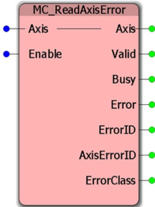
This Function Block reports axis alarms and warnings not related to the PLCopen Function Blocks. The ErrorClass output designates the source of the alarm or warning. The AxisErrorID output contains the error code.
