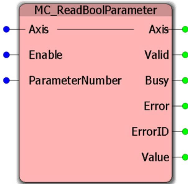
This Function Block reads the value of an axis specific boolean parameter and is for controller-side parameters only. For amplifier side parameters, refer to [Y\\_ReadDriveParameter](#).
