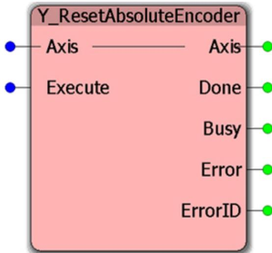
This Function Block clears absolute encoder alarms caused by battery power loss, cable disconnection, etc. This function block is equivalent to the Fn008 servo amplifier function, which can be performed from the front panel of an SGDh amplifier or via SigmaWin, or via the MPiC controllers webserver page.
