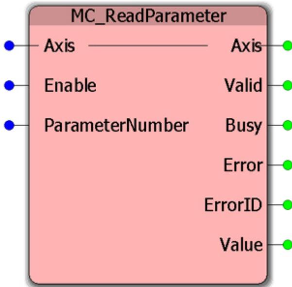
This Function Block returns the value of an axis-specific controller side parameter. For amplifier side parameters, refer to [Y\\_ReadDriveParameter](#).
