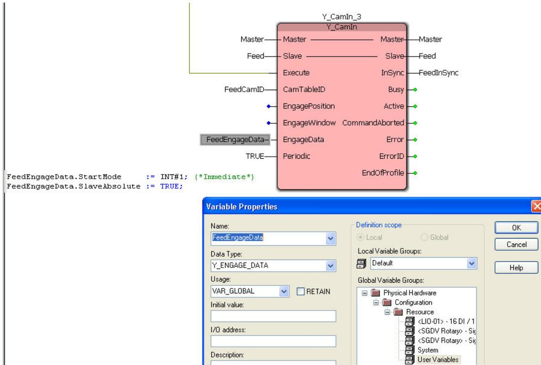
The diagram shows the Y\_CamIn\_3 function block with the following inputs and outputs:
