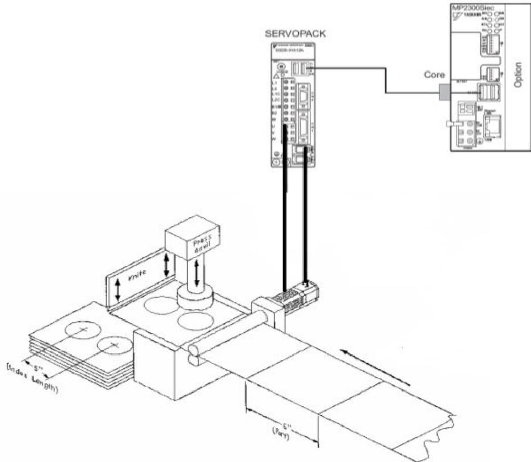
Feed to length application for a punch press
