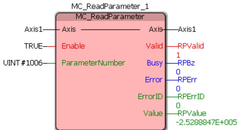
Instance of `MC_ReadParameter` reading non cyclic actual position of an axis
