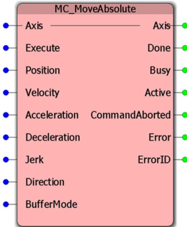
This Function Block commands a controlled motion to the specified absolute position.
