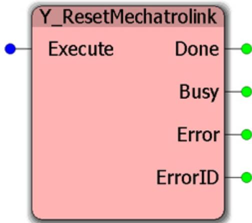
This function block resets the MECHATROLINK network. Nodes are temporarily disconnected from network and rediscovered afterward. This function is identical to the web interface's "Reset ServoNet" button.
