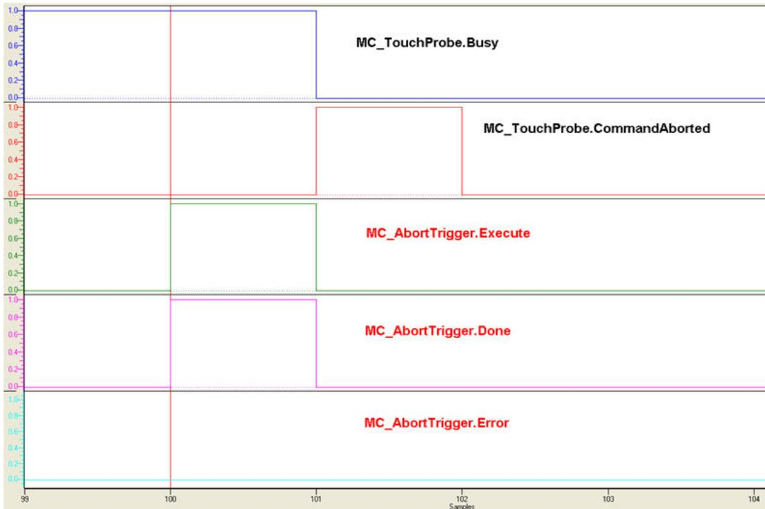
Timing Diagram for MC\_AbortTrigger
