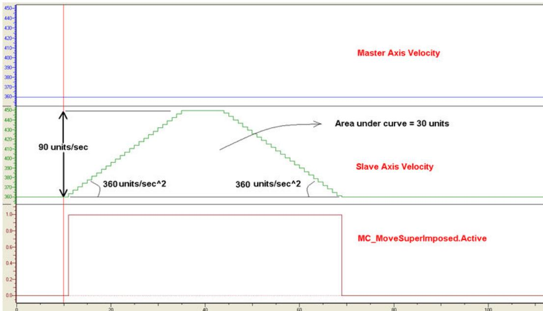
30 degree adjustment made while motion was continuing.
