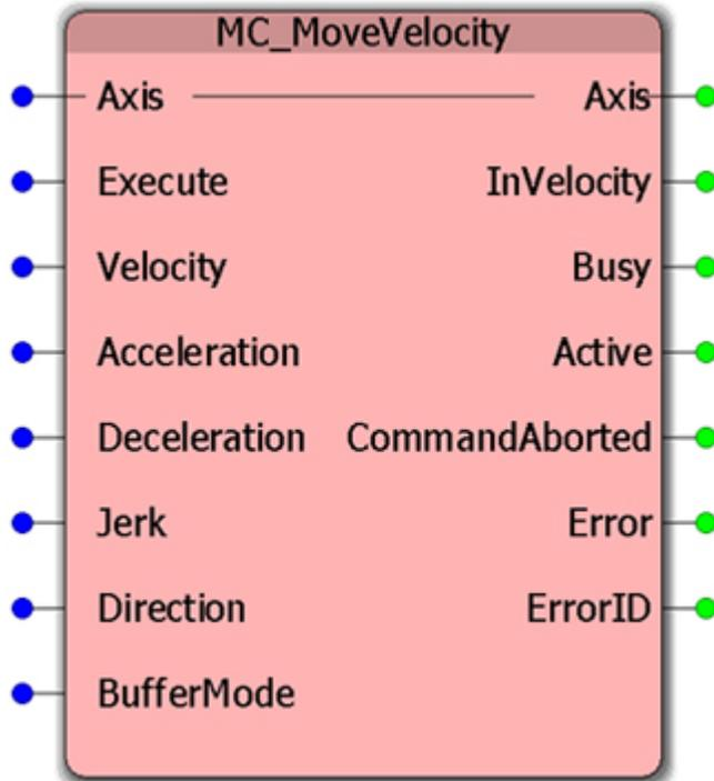
This Function Block commands a never ending controlled motion at the specified velocity.
