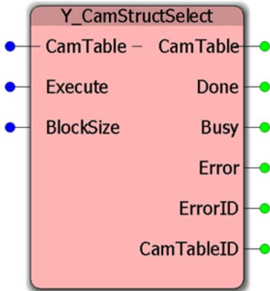
This function block loads a cam table from the application memory area to the motion memory area and returns a CamTableID to be referenced when activating the Cam function.
