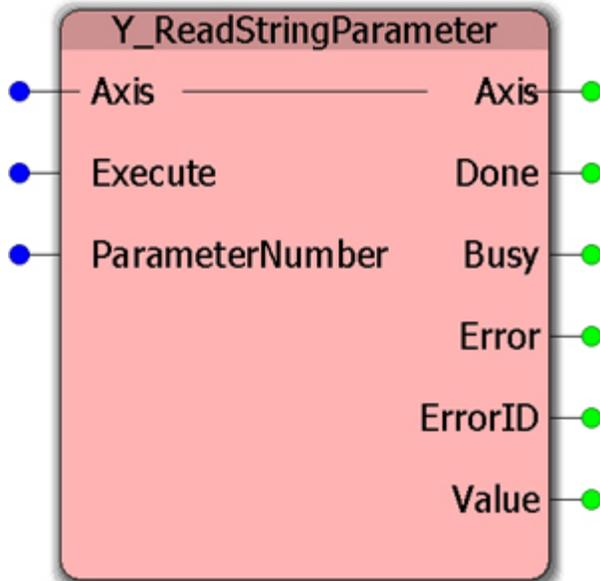
This Function Block returns the string value of an axis-specific parameter.
