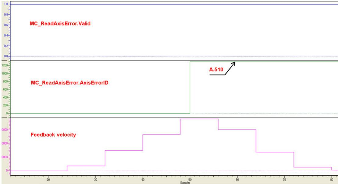
Timing diagram for an overspeed condition reflected in MC\_ReadAxisError
