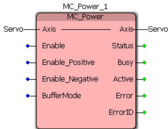
Initializing an axis and using MC\_Power to enable the axis
