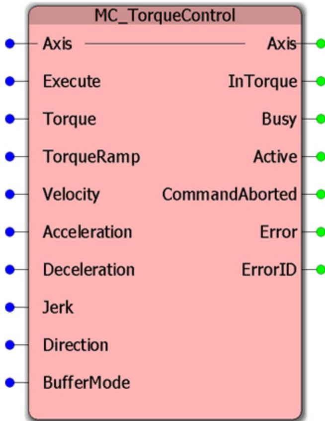
This function block continuously exerts a torque or force of the specified magnitude. This magnitude is approached using a defined ramp (TorqueRamp), and the Function Block sets the InTorque output if the commanded torque level is reached. This function block is applicable for force and torque. When there is no external load, force is applicable. Positive torque is in the positive direction of velocity.
