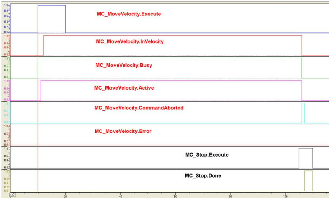
Timing Diagram for MC\_MoveVelocity
