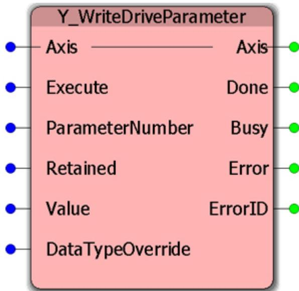
This Function Block writes the specified parameter to the drive or amplifier of the specified axis. To transfer a copy of all parameters from the controller to the amplifier, use [Y\\_WriteParameters](#).
