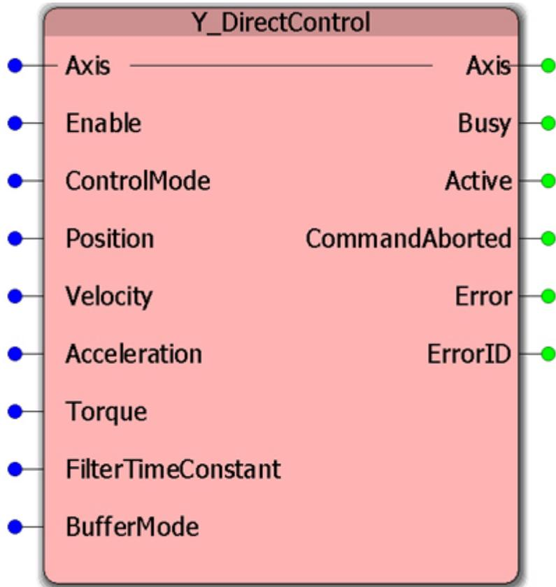
This block allows direct access to any of three possible control modes available on the specified axis. Y\_DirectControl makes it possible to perform open loop velocity control for winding applications. In position mode, the IEC application program can apply an algorithm to directly command the position at every scan.
