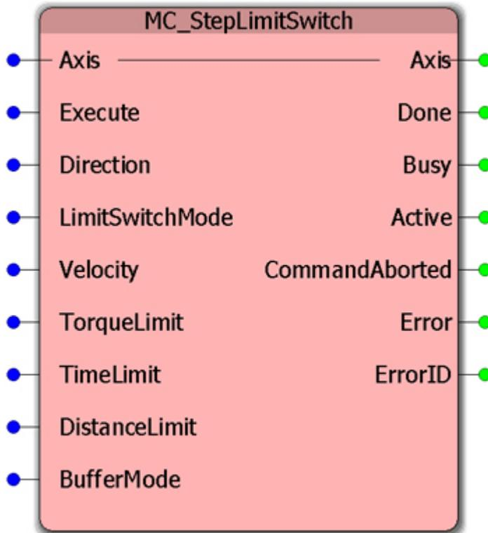
This function Block performs a homing function by searching for a limit switch. Logic is built-in to account for cases in which the limit is already hit. See the example below.
