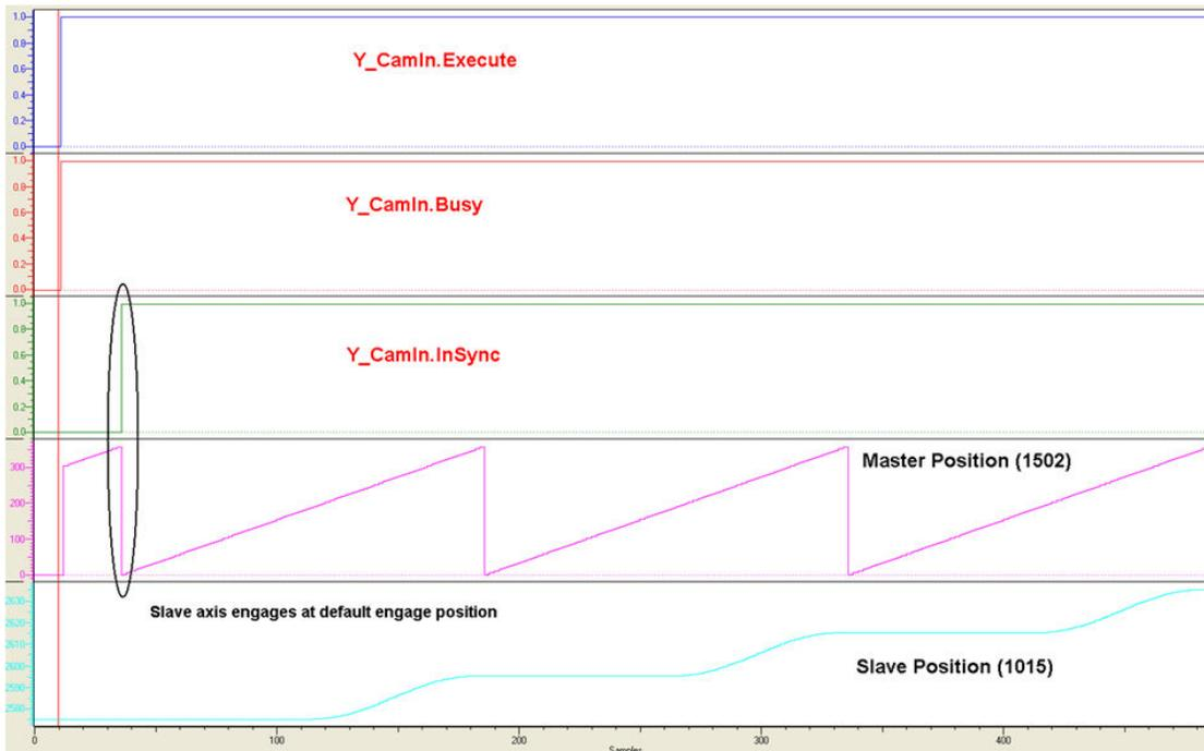
Notice that the function block executed before the actual master and slave started camming. This allows the Y\_CamIn function block to be placed in a slower application task while the motion task running at the MECHATROLINK or dual port RAM update interval monitors for the EngagePosition.
