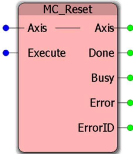
This function block will reset axis related alarms on either the controller or amplifier side.
