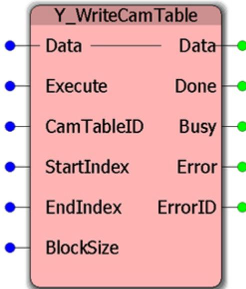
This Function Block copies cam data from the application program memory into the motion memory.
