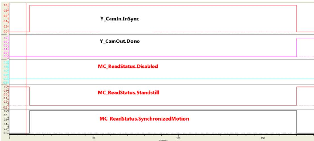
Timing diagram showing the outputs of MC\_ReadStatus before, during and after a camming operation
