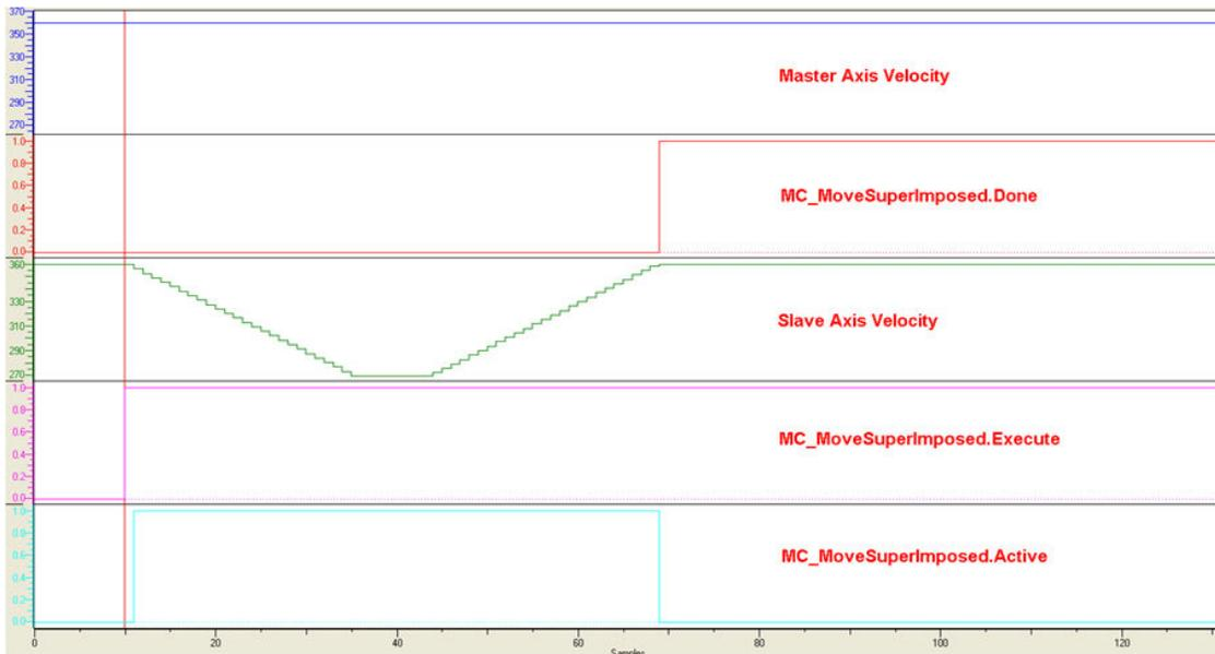
Timing diagram for MC\_MoveSuperImposed.
