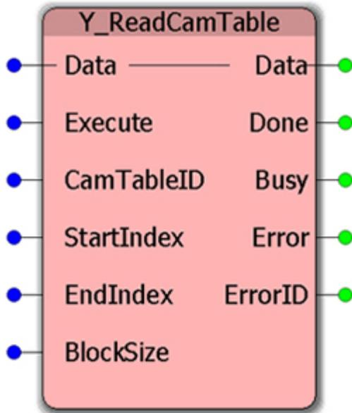
This Function Block copies a cam table from the motion memory into the application program memory.
