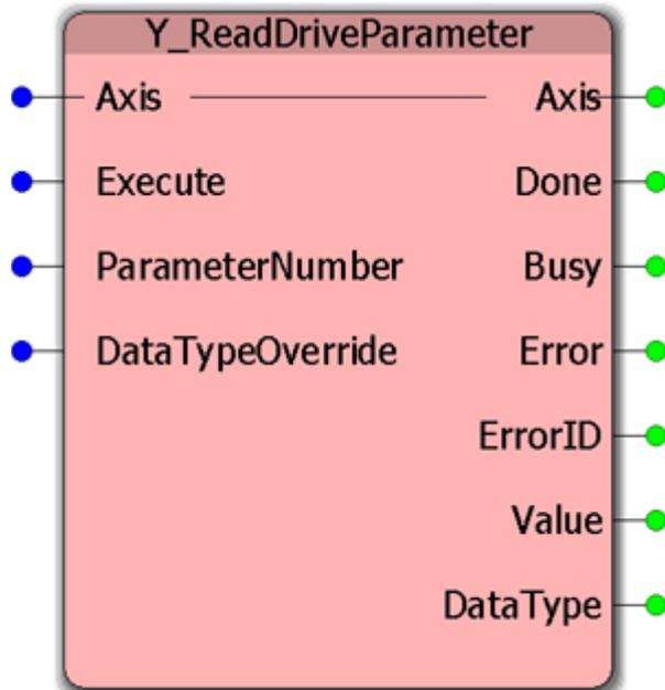
This Function Block reads the specified parameter from the drive or amplifier of the specified axis. To read a controller side axis parameter, use [MC\\_ReadParameter](#).
