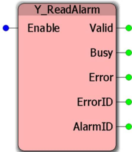
This Function Block reports controller-specific alarms that are not axis related. The Function Block [Y\\_ClearAlarms](#) clears alarms reported by this block.
