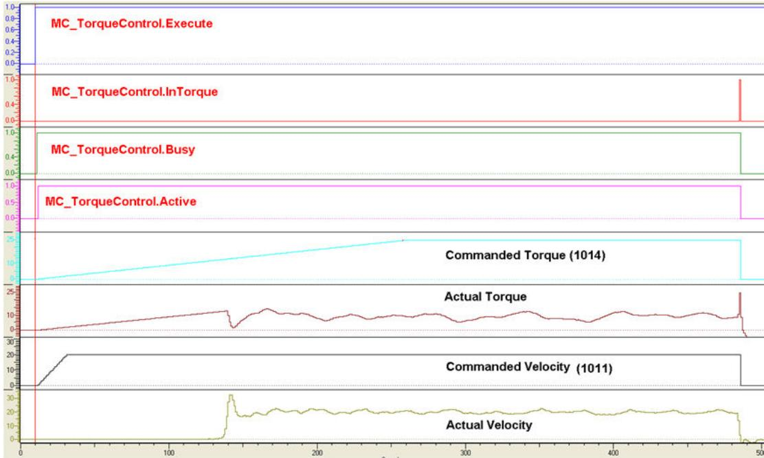
Example of MC\_TorqueControl being applied to move an axis to a hard stop
