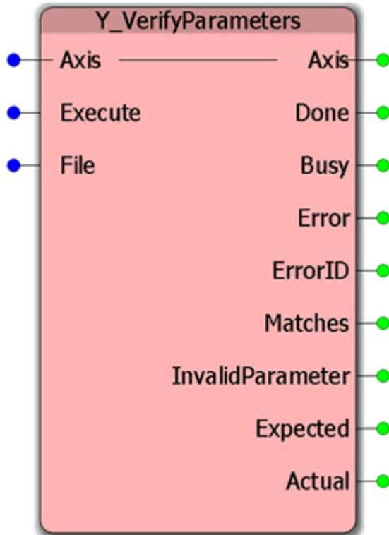
This Function Block compares the current parameters in the drive with the parameter file stored in the controller via the MotionWorks IEC Hardware Configuration.
