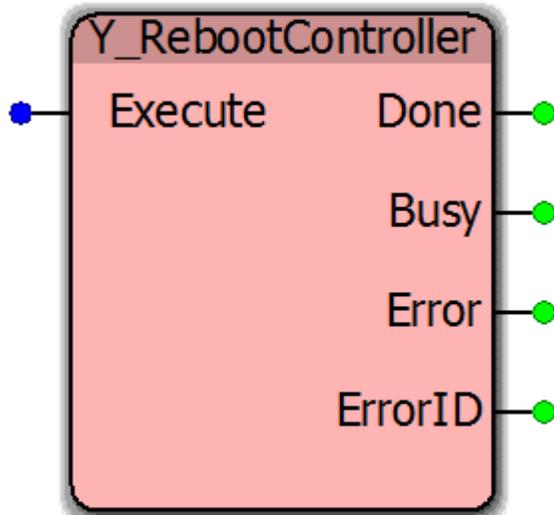
This function block reboots all controller processes, and reinitializes the MECHATROLINK network. Nodes are temporarily disconnected from network and rediscovered afterward. This function block was introduced in firmware version 2.5 for use with the MP2600iec controller and will execute on all other controller models. The application is similar to Y\_ResetMechatrolink, which is not supported on the MP2600iec. Resetting an option style amplifier causes its option card to reboot.
