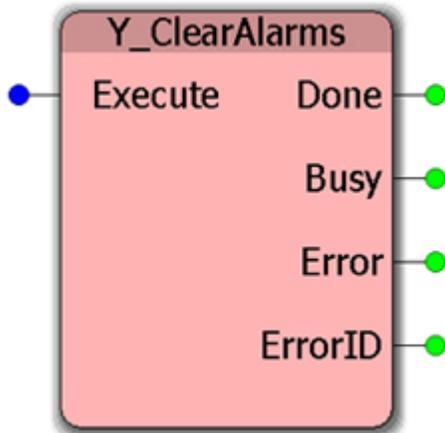
This Function Block clears controller based alarms that are not axis specific. To clear axis related alarms, use [MC\\_Reset](#).
