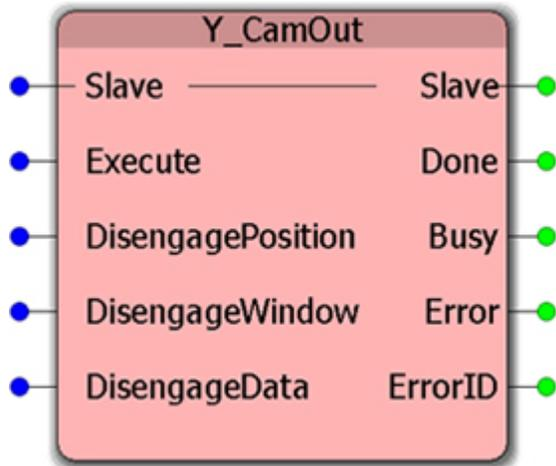
This Function Block disengages a Slave axis from its Master axis when the master is at the DisEngagePosition.
