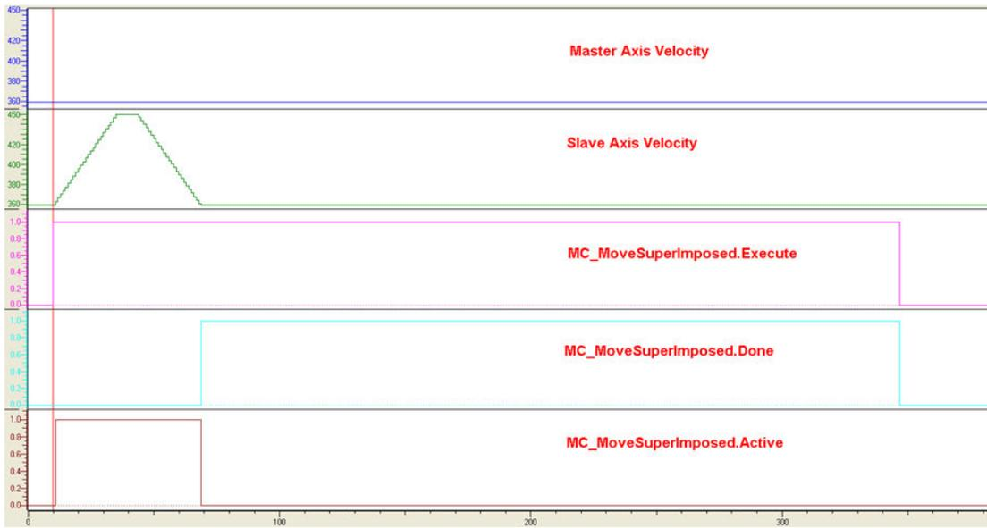
Timing diagram for MC\_MoveSuperImposed.
