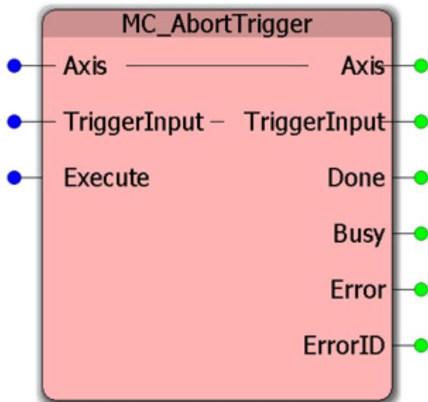
The Function Block aborts function blocks which are associated with trigger events (e.g. [MC\\_TouchProbe](#)).
