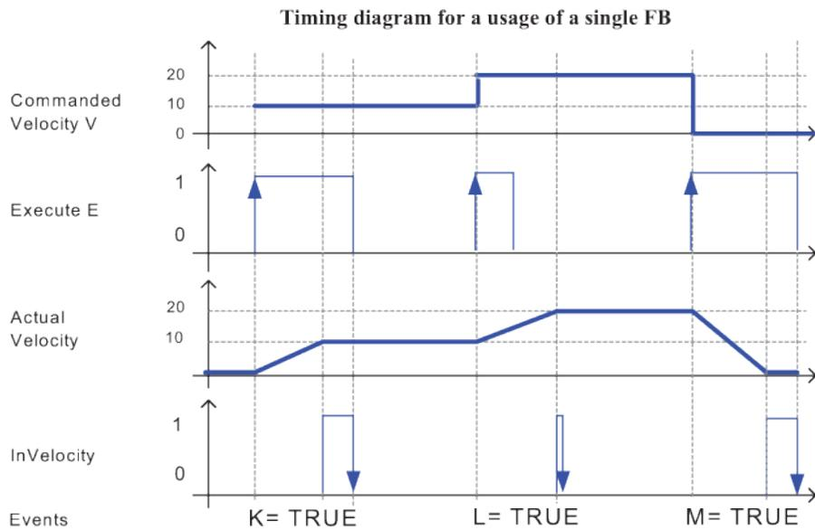
Note: The second InVelocity is set for only one cycle because the Execute has gone low before the Actual Velocity equals Commanded Velocity.
