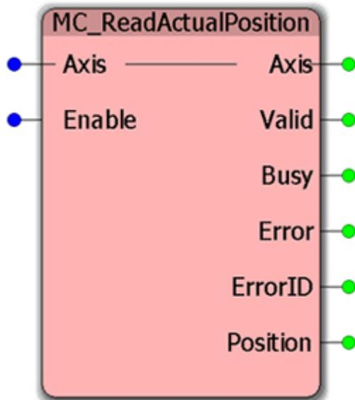
This Function Block returns the actual position of the axis in user units as configured in the Hardware Configuration.
