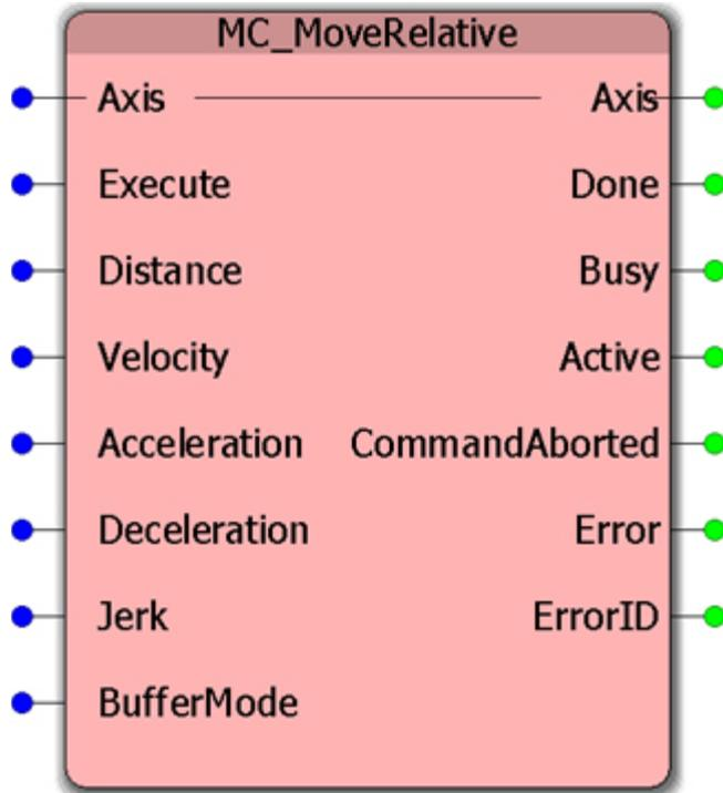
This Function Block commands a controlled motion of the specified distance relative to the commanded position at the time of the execution.
