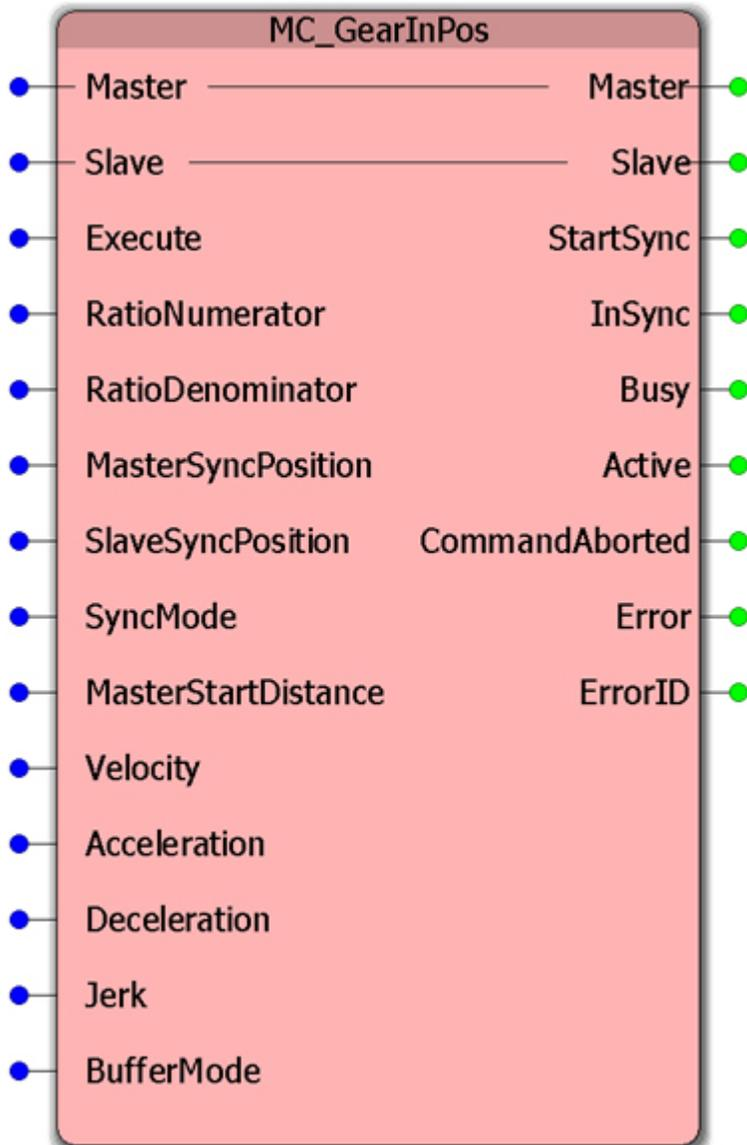
This Function Block commands a gear ratio between the master and slave axes. Position synchronization is achieved over a defined region of travel for both master and slave.
