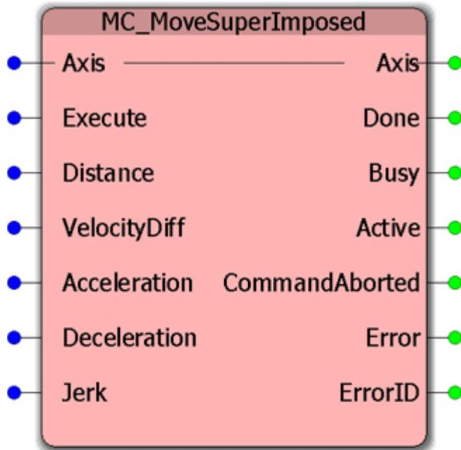
This Function Block commands a controlled motion of the specified relative distance additional to an existing motion. The existing Motion is not interrupted, but is superimposed by the additional motion.
