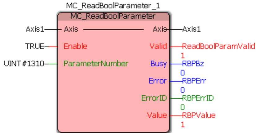
Instance of `MC_ReadBoolParameter` reading boolean controller parameter 1310. In this case controller parameter 1310 is enabled (`RBPValue = 1`).
