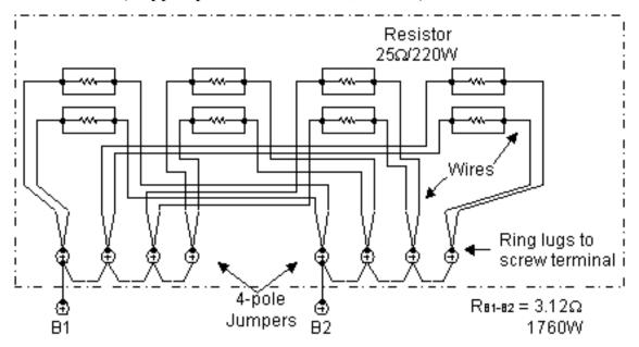
• Without the jumpers, this is essentially the same as wiring two JUSP-RA04 units.
