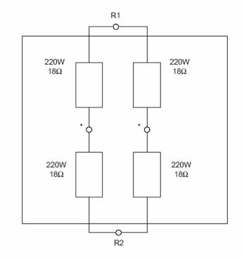
\*: These use terminal in parts hidden by the terminal block cover. These terminals should not be connected to from the outside.
