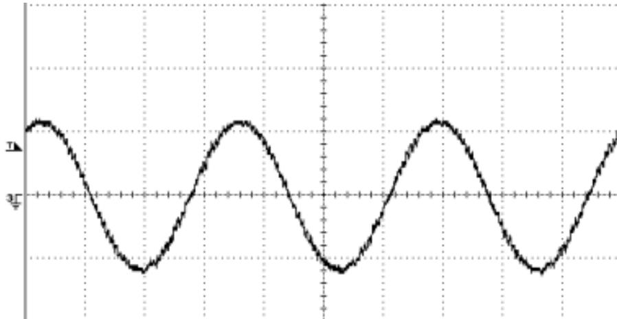
Eventually you get a sinusoidal current waveform albeit with some jagged up and down transitions as the voltage pulses start and end.
