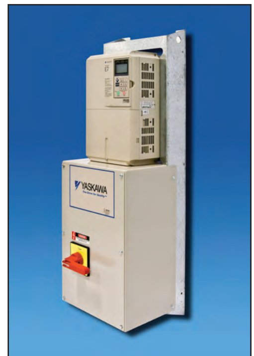
Figure 1. The obvious advantage that VFDs offer over soft starters is the ability to control motor speed. Depending on the application, lowering motor speed by 20% could reduce energy use by as much as 50%.
