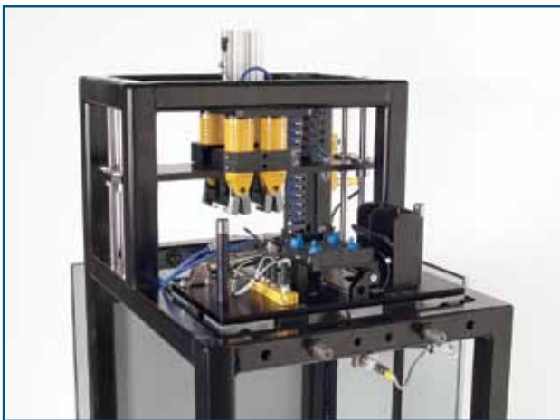
Punch Press Degater w/ Interchangeable Part Nests and Heated Cutting Steel.
