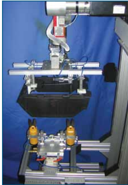
Rotary Degate Station reduces number of cutters and blades needed.
