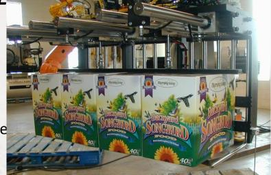
Solid stainless steel fingers are spaced to allow the gripper to be positioned between in-feed conveyor rollers
