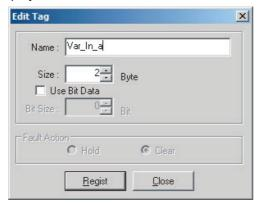
**5** Enter the variable name directly into the *Name* Box. (Example: *Var\_In\_a*)
