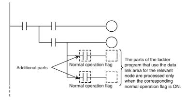
• You can use MC - MCR instructions and JMP instructions to process data only when the data links are operating normally as shown below.
