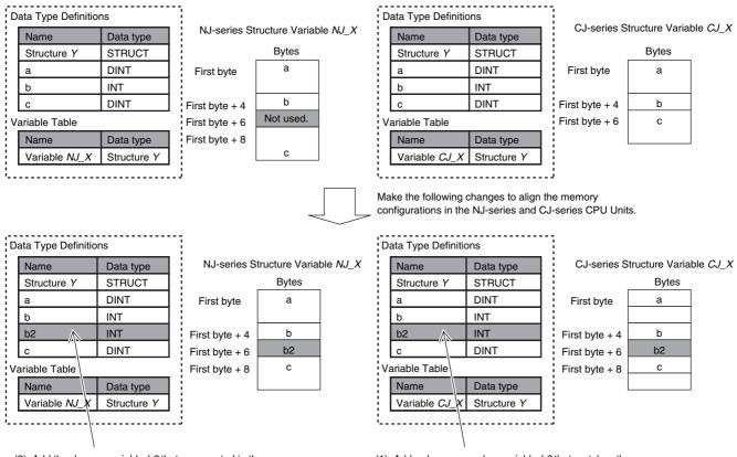
Add a dummy member variable b2 that matches the unused memory location on the NJ-series CPU Unit.
