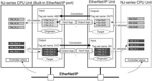
For communications between Controllers, the connection information is set in the EtherNet/IP Unit of the Controller that receives (consumes) the data (i.e., the originator).
