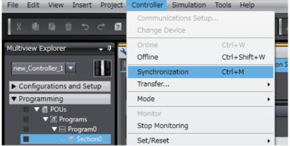
The Synchronization Window is displayed, and comparison of the user program and parameter settings between the Sysmac Studio and the Controller is started.
