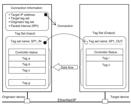
In this example, a connection is established with the originator's tag list with tags a to g (inputs), which are in a tag set called SP1\_IN, and the target's tag list with tags i and ii (outputs), which are in a tag set called SP1\_OUT.
