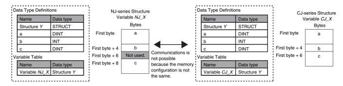
To align the memory configurations in the NJ-series and CJ-series CPU Units, offsets are set in the Sysmac Studio.
