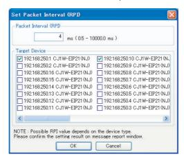
The percentage of the allowed tag data link bandwidth being used (Usage of Capacity) increases to 77.83% for devices 192.168.250.1 and 192.168.250.10, which indicates that the RPI is set to a higher speed for these devices' connections.
