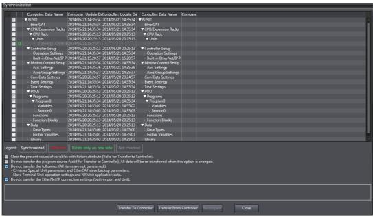
Clear the Do not transfer the EtherNet/IP connection settings (built-in port and Unit) Check Box and click the Transfer to Controller Button.
