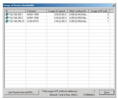
The *Usage of Capacity* (without multicast filter) column will show the percentage of the allowed tag data link bandwidth being used, and the *Mbit/s* (without multicast filter) column will show the network bandwidth being used.
