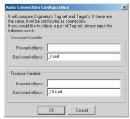
Input the ellipses and click the **OK** Button. Processing for automatic setting is started.
