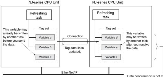
Data concurrency is not maintained unless you assign the same refreshing task for both the output and the input tags.
