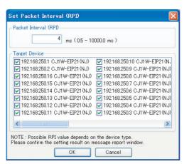
If the packet interval for all connections has been set to the same setting, the dialog box will show that the usage of capacity for the tag data link's allowable communications bandwidth is 76.17% and the fastest set value is 4 ms.
