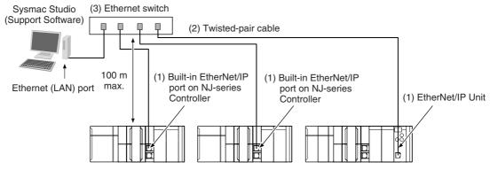
EtherNet/IP System Configuration Example
