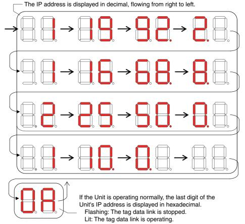
If an error occurs, the error code will be displayed alternately with the rightmost byte of the affected device's IP address. For details on error codes, refer to Section 13 Troubleshooting.
