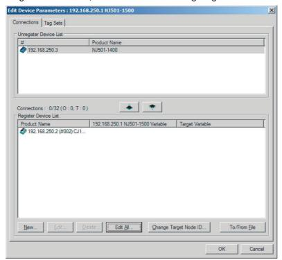
Target node IDs are assigned to the devices that are registered in the Register Device List.
