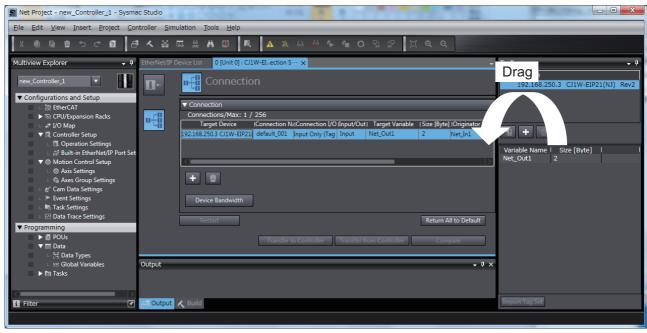
Specify Originator Variable and its Size [Byte] for the tag set Net\_Out1 added in step 5. Here, specify Net\_In1 for Originator Variable and 2 for its Size [Byte].
