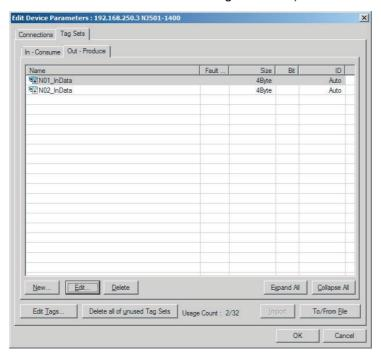
To place more than one input variable (input tag) imported from the Sysmac Studio into one tag set, you must delete the input tags that were registered. Select the tag set containing the variables you want to put into a tag set, then click the **Delete** Button. A confirmation dialog box is displayed to confirm that you want to delete the selected tag set and the tags contained in that tag set. You only want to delete the tag set, so click the **No** Button.
