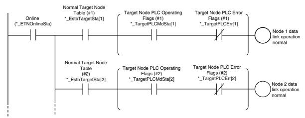
Programming Example 2 to Detect Normal Operation
