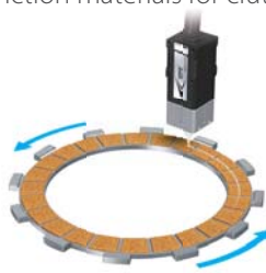
Profile inspection of friction materials for clutch
