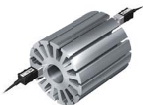
Thickness measurement of motor cores
