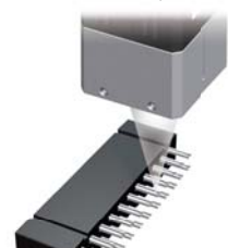
Coplanarity measurement of connector pins
