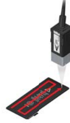
Flatness measurement of batteries
