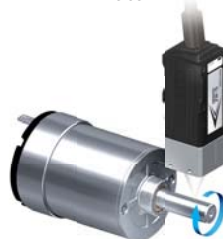
Eccentricity measurement of motor
