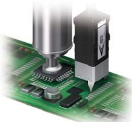
Z axis adjustment of chip mounter
