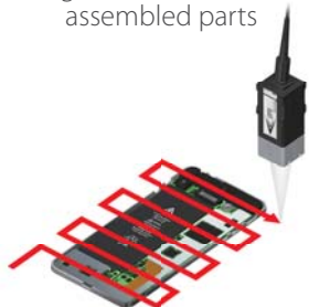
Height measurement of assembled parts
