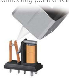
Operation inspection of connecting point of relay
