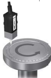
Flatness measurement of transmission parts
