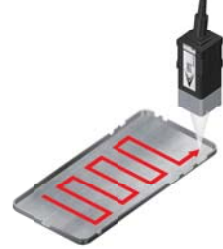
Flatness measurement of cases
