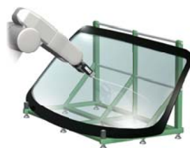
Curvature measurement of glass surface
