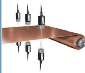
Thickness measurement of battery sheets
