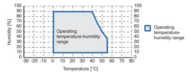
The ambient operating temperature specifications do not depend on the mounting angle, orientation or display size. • Store the Industrial Monitor within the following ambient temperature and humidity ranges.
