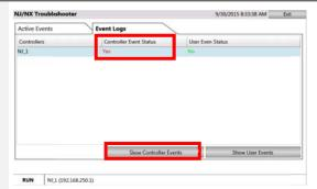
[Controller Event Logs Page] is displayed. A list of controller event logs is displayed. Select the controller event log that you want to check, and click the "Show Detail" button.
