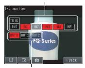
Output Signals (OUT0, OUT1, and OUT2)
