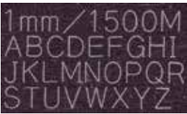
Workpiece: Aluminium Letter height: 1mm
