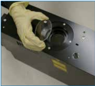
The double glass cover makes it easier and safer to change the glass.
