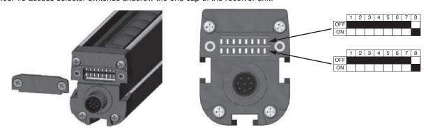
Note: There are two lines of dip switches in each transmitter and receiver. The settings must be done for both lines. Change the setting of the dip-switch and close the cap again. The light grid can now be reconnected to the power supply.
