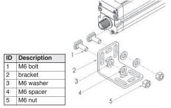
Note: Shipments contain a different quantity of brackets, depending on the length of the light grid. Longer light grids contain a higher number of brackets, following the rule of one bracket every 400 mm.
