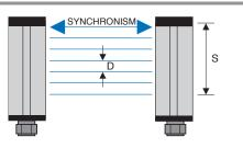
S: Sensing area D: Beam axis pitch
