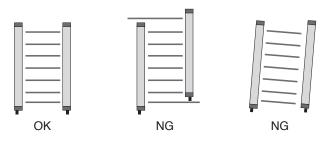
If several light grids are installed close to each other, interference of the light grids must be avoided. In this case the assembly should be carried out as follows:
