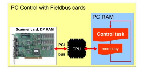
EtherCAT: MAC is PCI Bus master, data is provided by DMA directly to PC RAM: CPU relieved more performance
