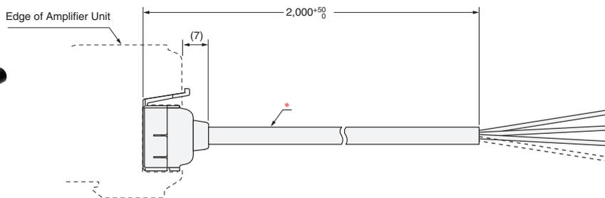
\* E3X-CN11: 4-dia. cable with 3 conductors, Standard cable length: 2 m (Conductor cross-section: 0.2 mm<sup>2</sup> (AWG24), Insulator diameter: 1.1 mm)
