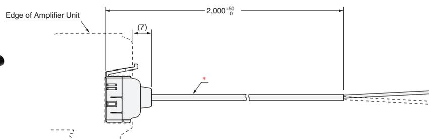
\* E3X-CN12: 2.6-dia. cable with 1 conductor, Standard cable length: 2 m (Conductor cross-section: 0.2 mm<sup>2</sup> (AWG24), Insulator diameter: 1.1 mm)
