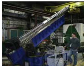
Convertible Test System 20,000 lb load - 100" CC
