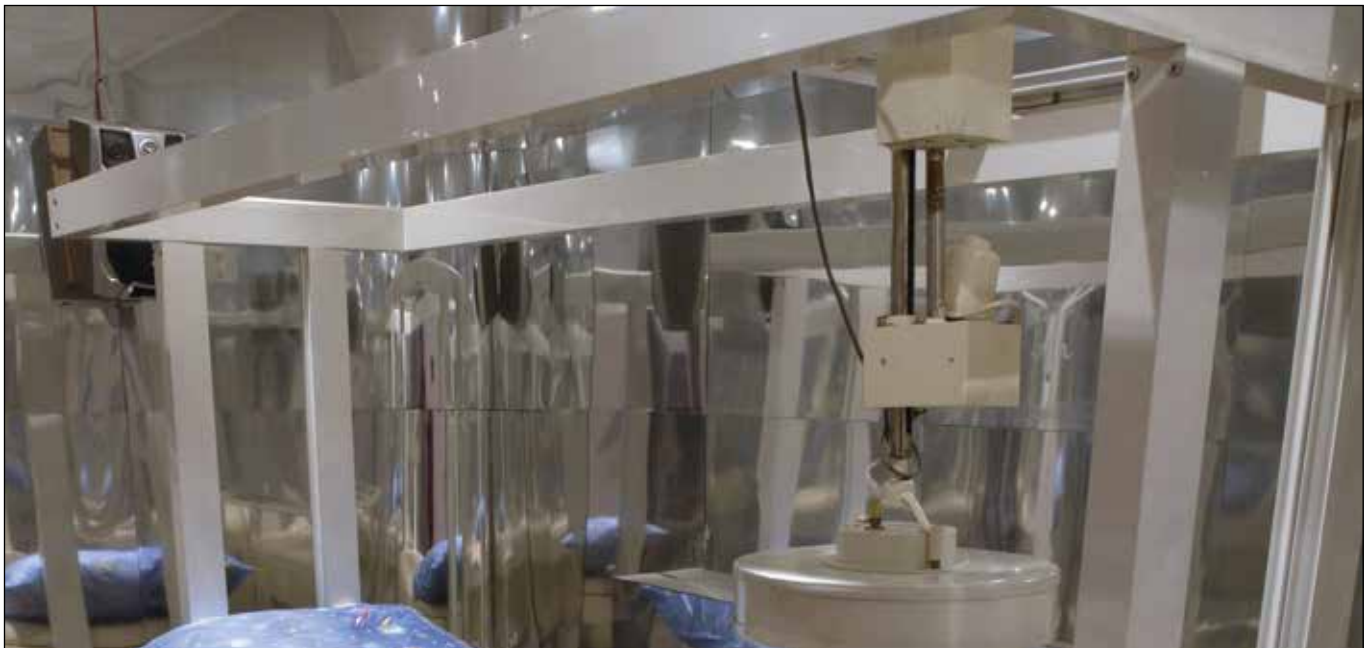
Nook Linear Shafting and Bearings used to guide a loader for medical waste processing.
