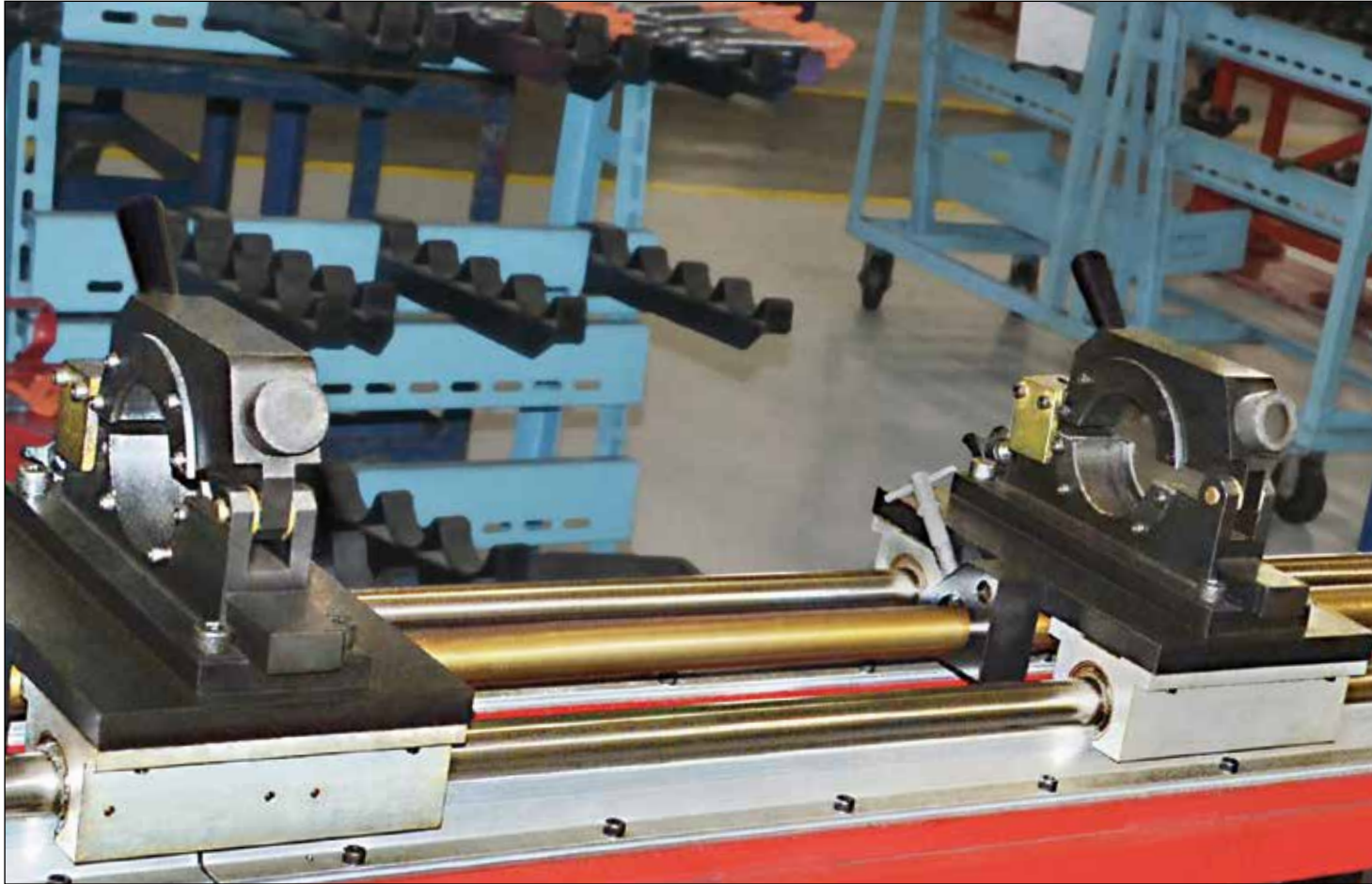
Nook slide rail system used as a steady rest for a large diameter CNC machine.
