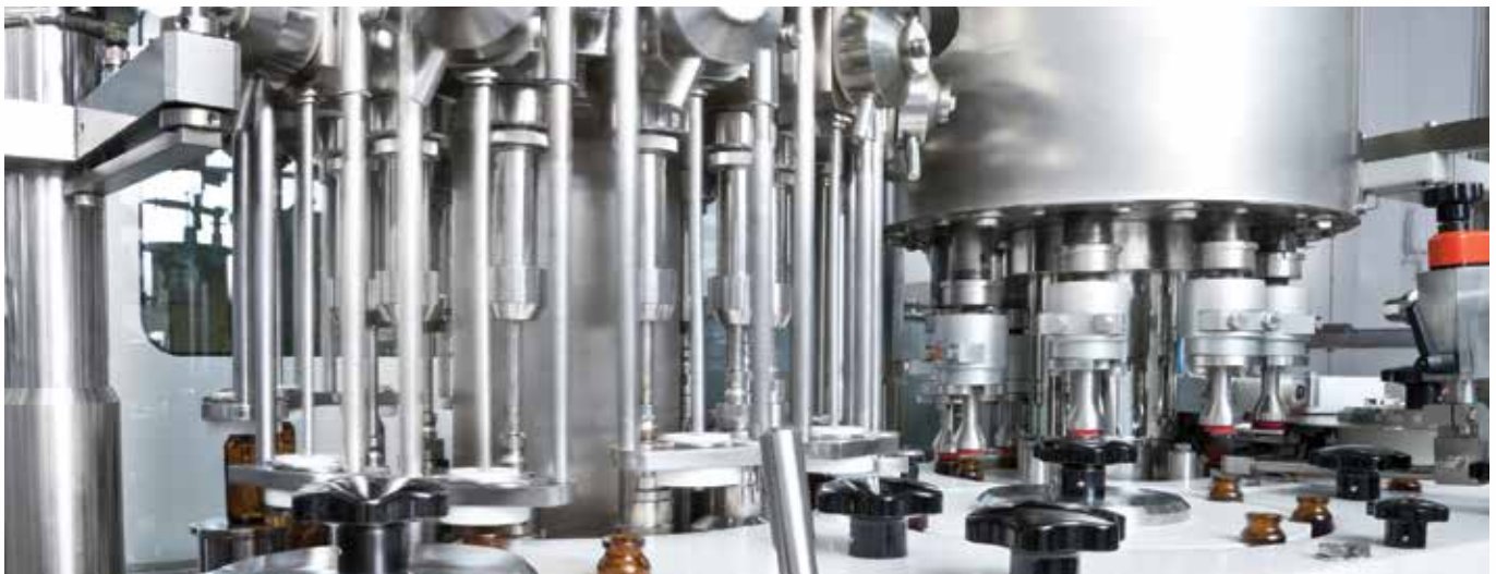
Nook linear shafts used to guide a bottle filler application.
