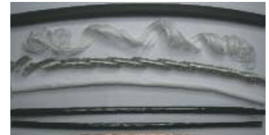
Test samples of CFROBOT-037 were taken at 250,000, 1.5 million and 3 million movements. The CFROBOT-037 cables has no sign of damage even after 3 million torsional movements of \pm 270^\circ .
