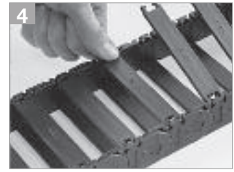
4 To close crossbars: push down on crossbar with thumb until it snaps into place
