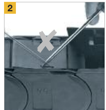
2 Release only one side to open the lid
