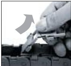
Opening the zip – pull the lid at the end of the chain upward and outward
