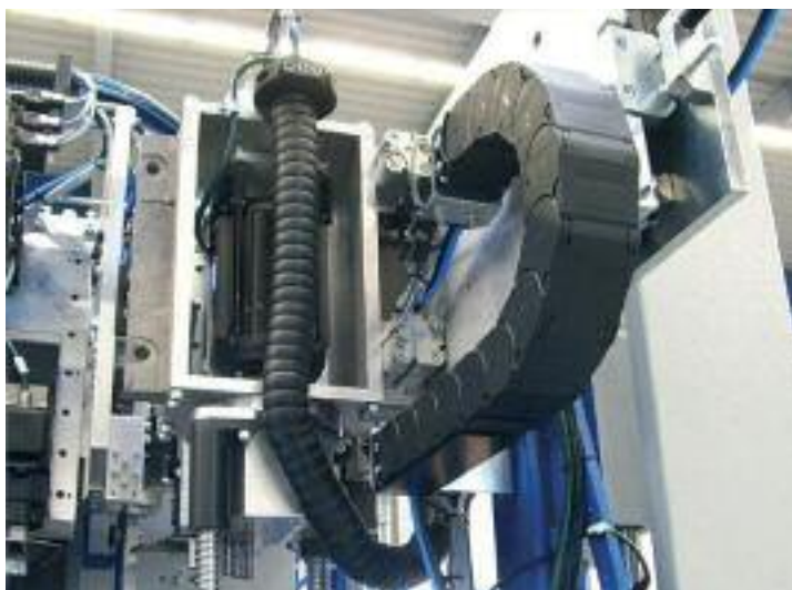
igus® E2 Energy Tube and Triflex® R in a processing machine
