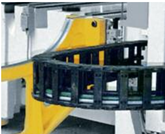
Special case: Side-mounted, unsupported - undercut design offers stability
