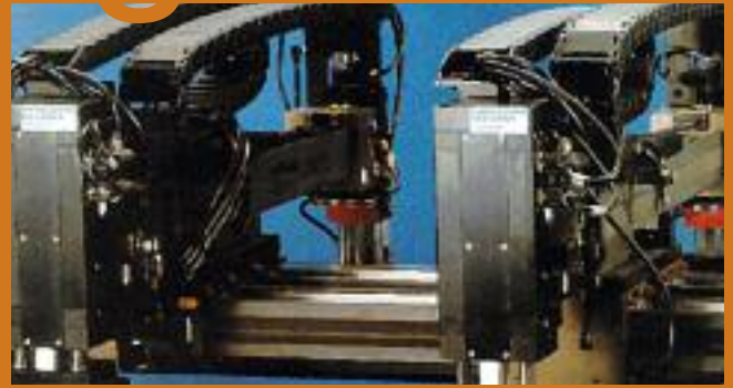
Automatic PC board component insertion unit with igus® Zipper Series 15. Accelerations up to 328 ft/s 2 (100 m/s 2 )
