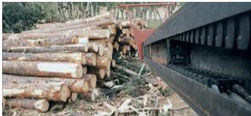
igus® Energy Chains® with hydraulic hoses in a tree-stripping machine
