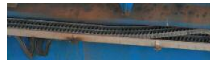
An igus® energy supply system with an approx. length of 82 ft in a stainless steel trough with middle band support.
