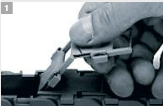
1 Zipp - upward . All lids fit like a "Zipper"
