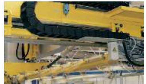
System E4 partially unsupported - please consult igus regarding this type of configuration.
