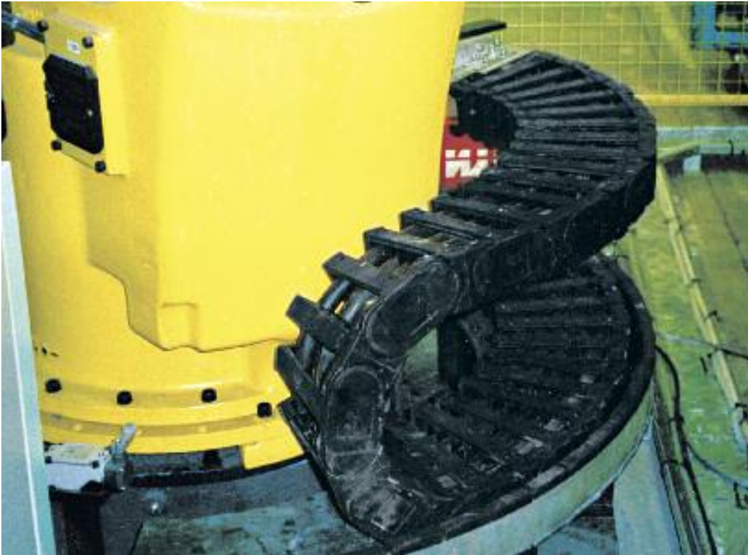
TwisterChain® for continuous industrial use on a buckling arm robot (for welding applications, rotary movement 420°)
