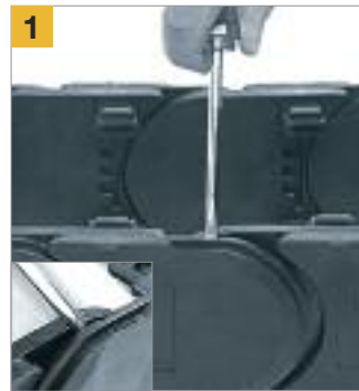
1 Remove crossbars, clips, and lids on two adjacent chain links. Guide the screwdriver into the slot between side links and release it by levering it and separate the Energy Chain®
