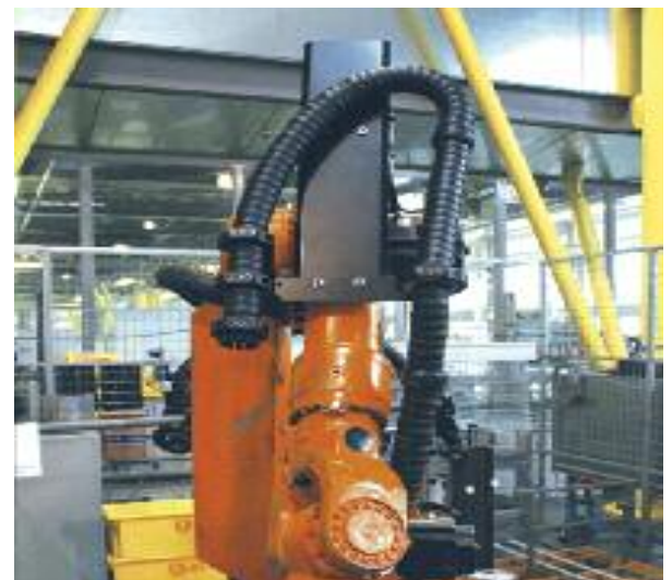
Integrated recuperating spring prevents loop formations
