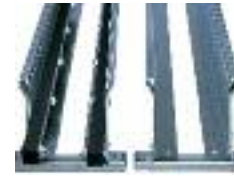
Left: Guide trough with glide bars
