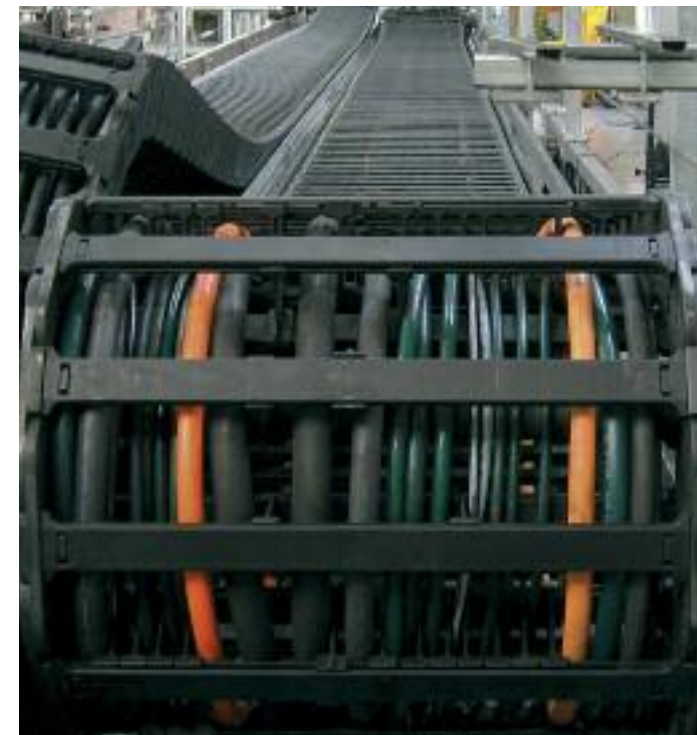
Actual test picture: Chainflex® cables were intentionally installed close together without adequate clearance to test their performance in a harsh application.
