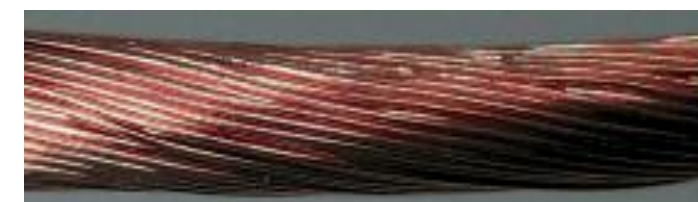
A close-up of the completely intact copper conductor. The inspection performed over the entire length shows that the conductor is still completely intact and does not have any individual wire breakages.
