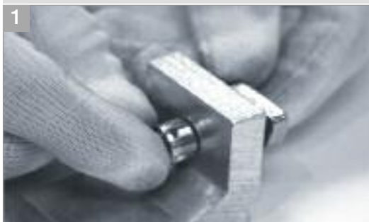
1 Pre-assemble heavy duty bracket and screw set
