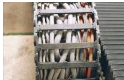
Corkscrewing: an effect of improper cable and hose placement in an Energy Chain®
