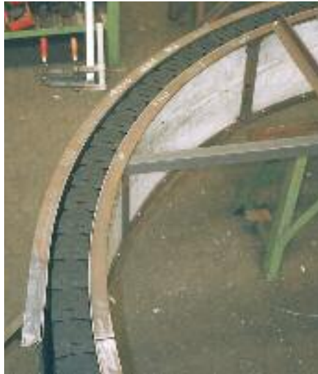
Guide troughs for rotary applications
