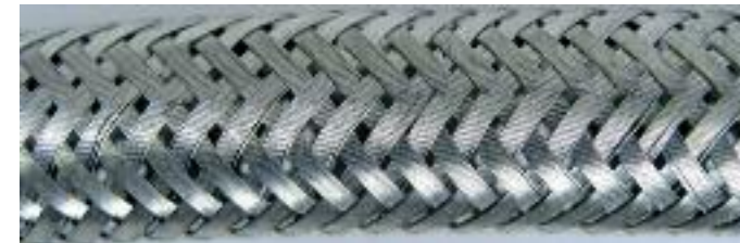
CF21.40.10.02.01.UL: after more than five million cycles, no shield wire breakages
