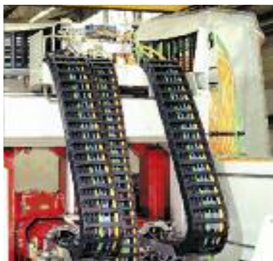
ReadyChain® with combined motions on tooling machines
