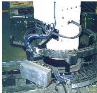
Spiral and rotary movement TwisterChain®
