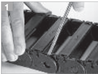
1 Separating chain sections: insert screwdriver between two links. Twist until pin disengages from bore; pull sections apart
