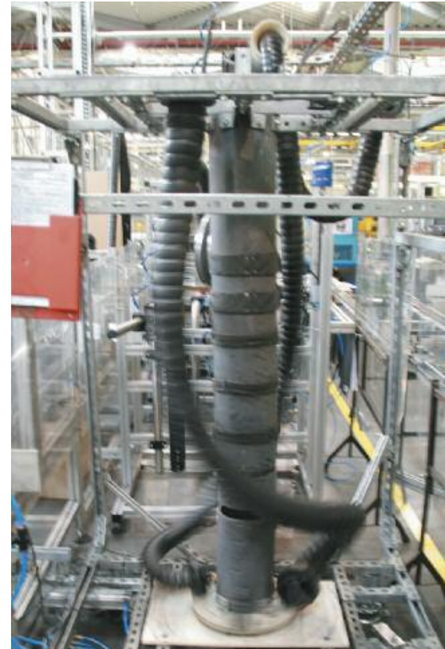
igus® test lab: The cables were tested in movements of \pm 270^\circ .
