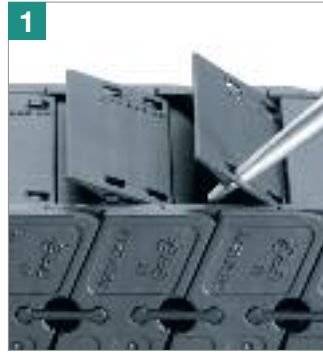
1 Lever with screwdriver ...
