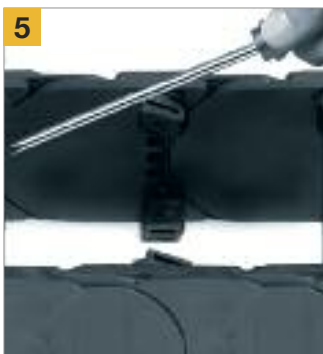
5 Assemble clips (for Energy Chains with crossbars every other link) - push down and snap in using a screwdriver
