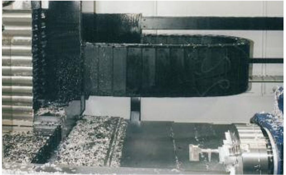
System E4 Energy Tube in direct chip area E4/light
