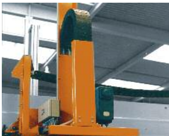
U-shaped supported Energy Tube for high lateral acceleration
