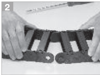
1 Separating chain sections: insert screwdriver between two links. Twist until pin disengages from bore; pull sections apart
