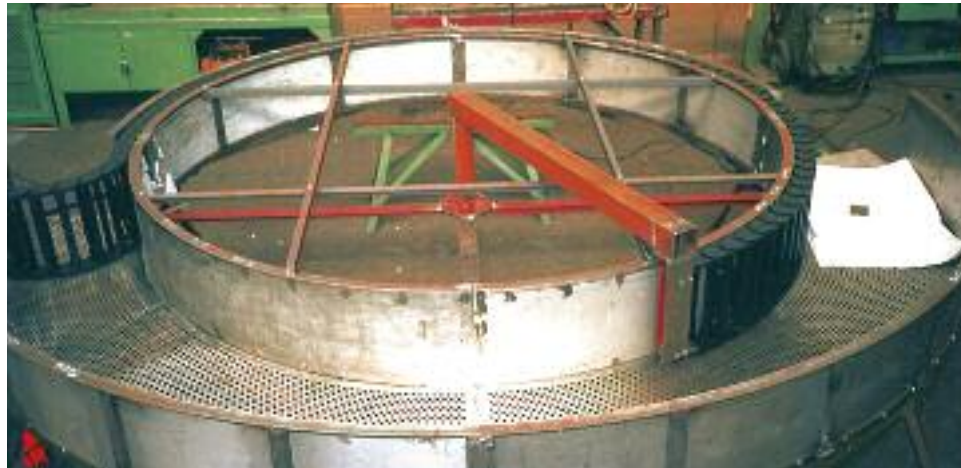
Rotary motion with RBR; diameter 236" (6000 mm); Series 50 with RBR; the inner ring rotates
