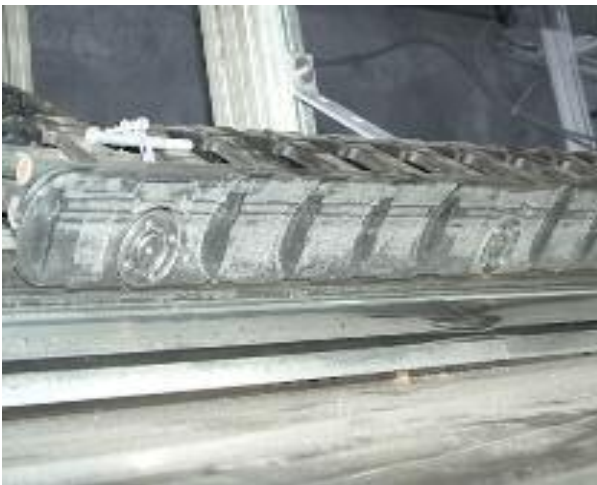
Test - Glide strips minimize wear after 1,653,187 cycles, 2,672 miles (4,300 km)
