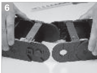
6 6. Twist until pin disengages from bore; pull sections apart
