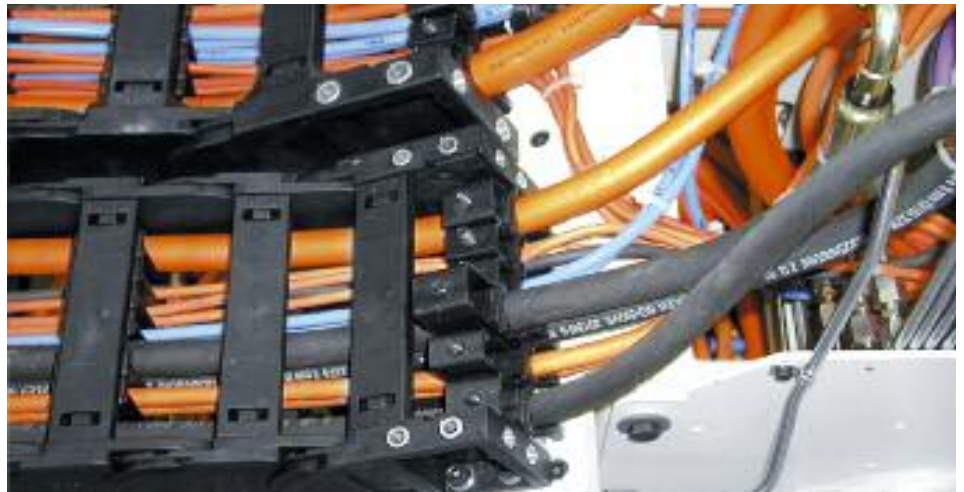
Chainfix strain relief with KMA brackets; used here for cables and hoses
