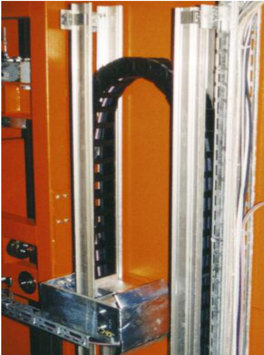
Energy Chain® on the tower of the storage and retrieval unit for high-bay warehouses rolls off from one aluminum guide trough to the opposite one
