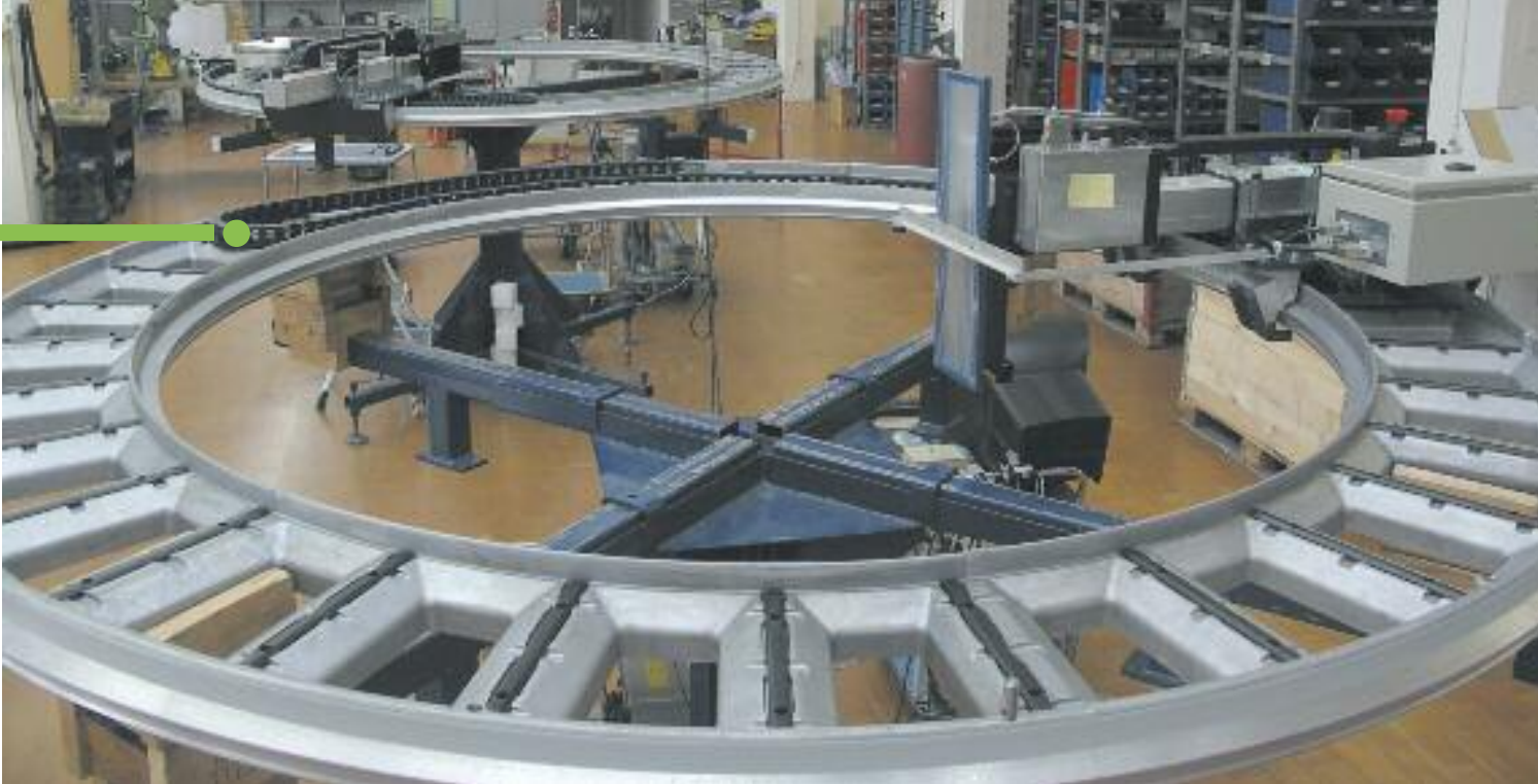
E2 mini Energy Chain®, RBR-version with reverse bending radius
