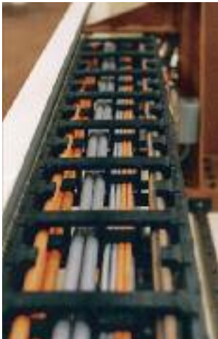
Neatly laid cables with igus® interior separation
