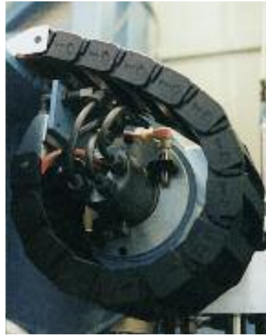
Rotary motion with a “standard” Energy Chain®
