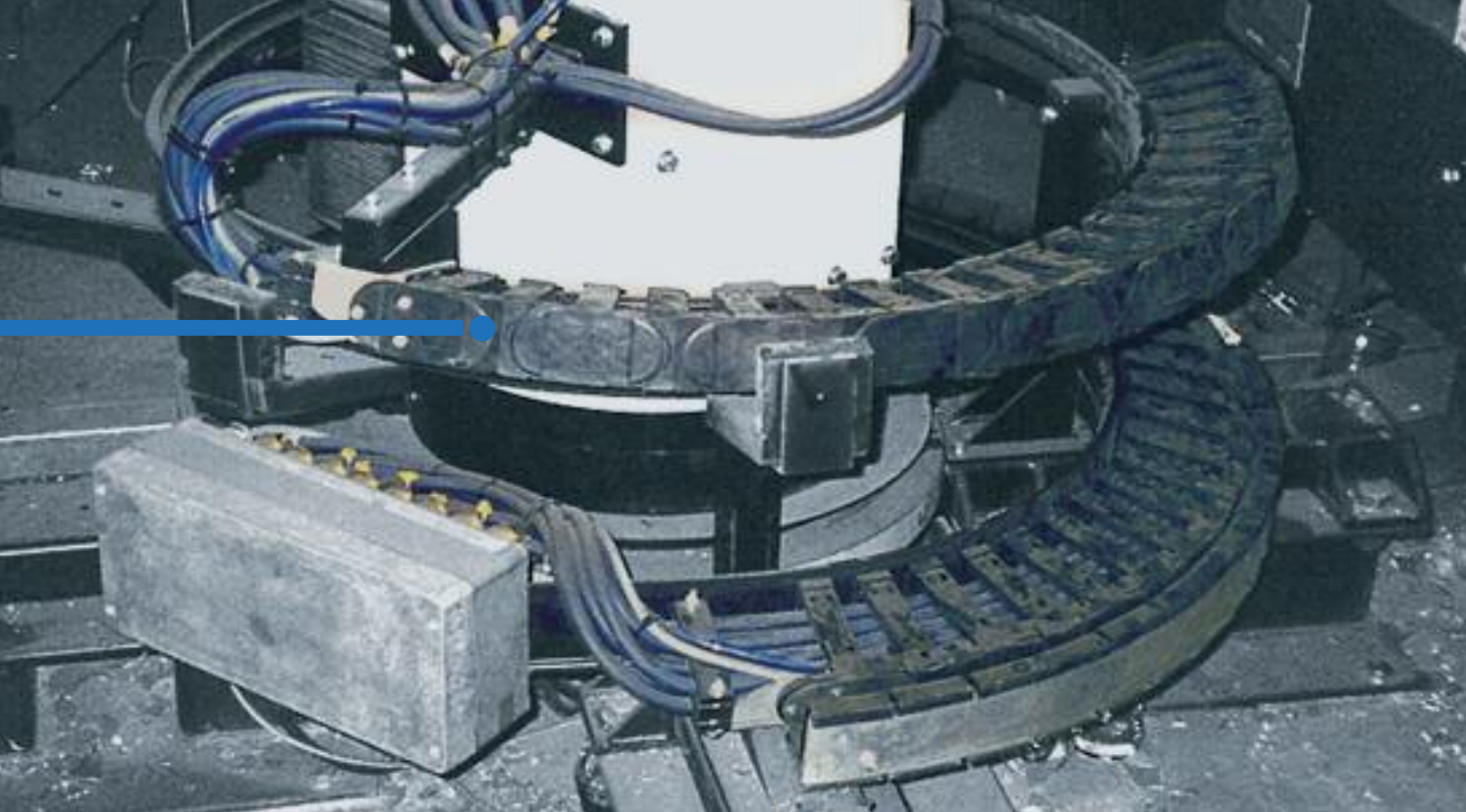
Combined spiral and rotary movement - igus® Series TwisterChain®
