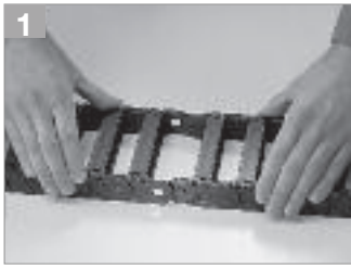
1 Joining chain sections: push sections together; angle one side until pin snaps into bore; repeat on other side
