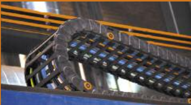
The Rol E-Chain ® Energy Chains ® require 75 % less drive power (gliding operation)
