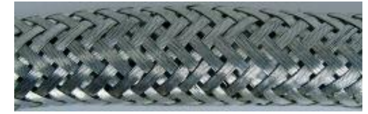
CF27-40-10-02-01-D: after more than five million cycles, no shield wire breakages
