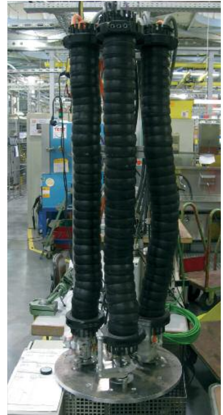
The "torsion test bench" especially developed according to the igus® standard
