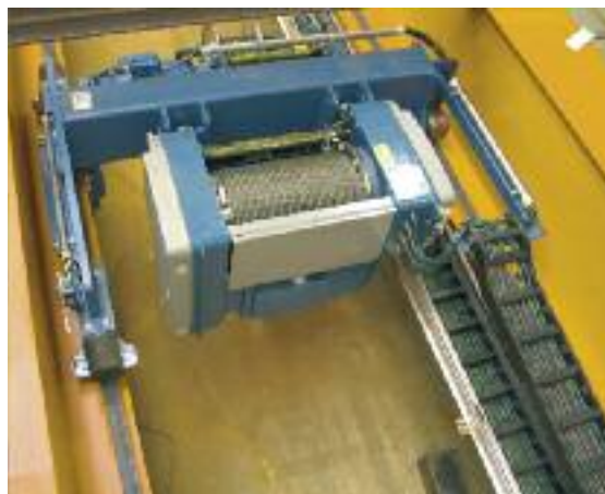
With the space-saving igus® E4 Polymer Energy Chains® the overall dimension for the installation for this crane system was considerably reduced
