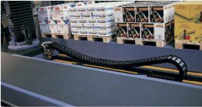
Example of unsupported with FL_B sag
