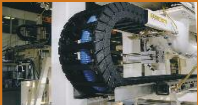
igus ® System E6 - High acceleration (8g) and ESD safety
