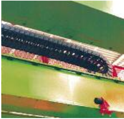
Unsupported application System E4, up to 164 ft/s (50 m/s) speed
