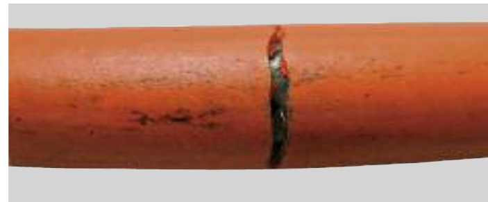
Test samples of cable jackets cracking with exposure to oils
