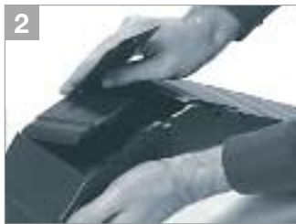
2 Bend Energy Tube to remove lid
