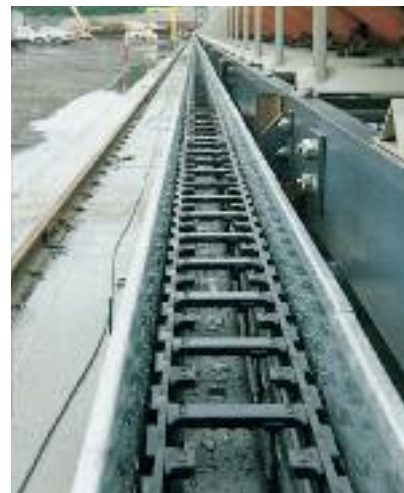
Conveyor belt in quarry. Travel distance of 587 ft (179 m), travel speed 220 ft/min. (67 m/min.) and fill weight 5.38 lbs/ft (8 kg/m)
