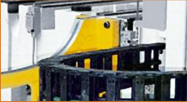
Unsupported, side-mounted application with Series E4/4 - higher stability due to "undercut-principle"
