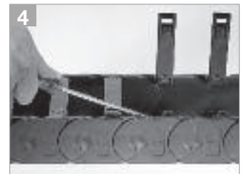
4 3. To close crossbars: push down on crossbar with thumb until it snaps into place
