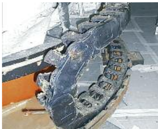
The robust link design allows also safety work in a dirty environment
