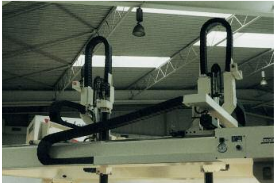
Standing application with support of the first chain links; R68 Energy Tube
