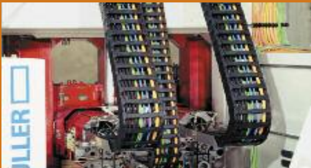
ReadyChain® with combined motions on tooling machines. Turnkey delivered with special parts for your machines
