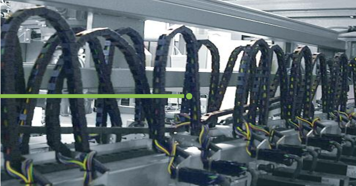
igus® E2 micro Energy Chains® are robust for standing applications
