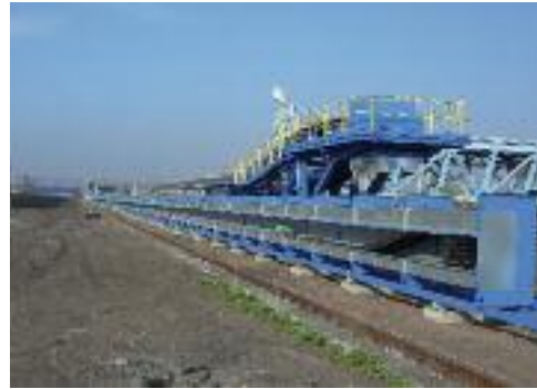
Longest igus® travel of 2,018 ft (615 m) with Rol-E-Chain and Chainflex® cables
