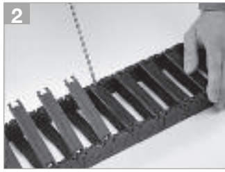
2 To open crossbars: press screwdriver into tab on top of link, lever screwdriver until crossbar opens
