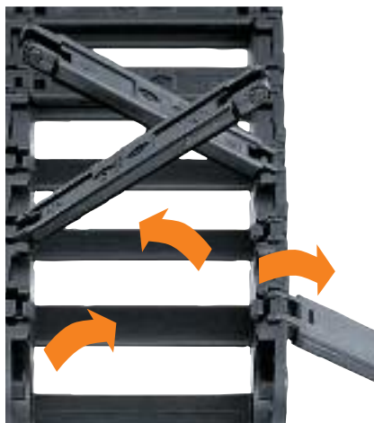
Special snap-open mechanism, choice of snap-open on left or right. Hinged crossbar can be swiveled by more than 180° on both sides
