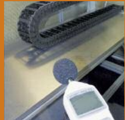
Noise level test inside an acoustic cabin
