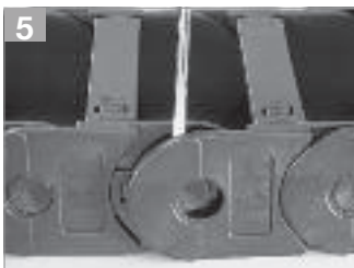
5 5. Separating chain sections: insert screwdriver between two links
