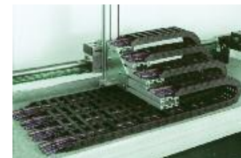
Example from iglus® test laboratory: continuous development and testing of Chainflex® round electrical cables
