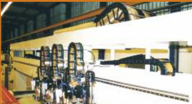
Extension links for E2 and E4 for large conduits up to Ø 9.84" (250 mm)
