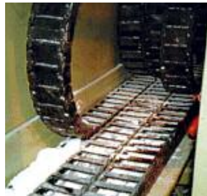
Energy Chains® side by side as individual or "multiband" Series "Zipper"
