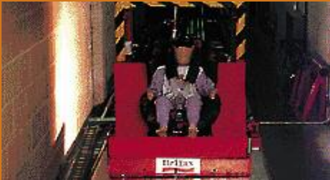
Crash test unit: 72 ft/s (22 m/s) and 2,572 ft/s 2 (784 m/s 2 ) acceleration for (36 m) travel
