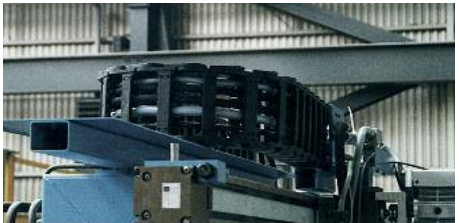
Energy Chain®, side-mounted, supported System E4
