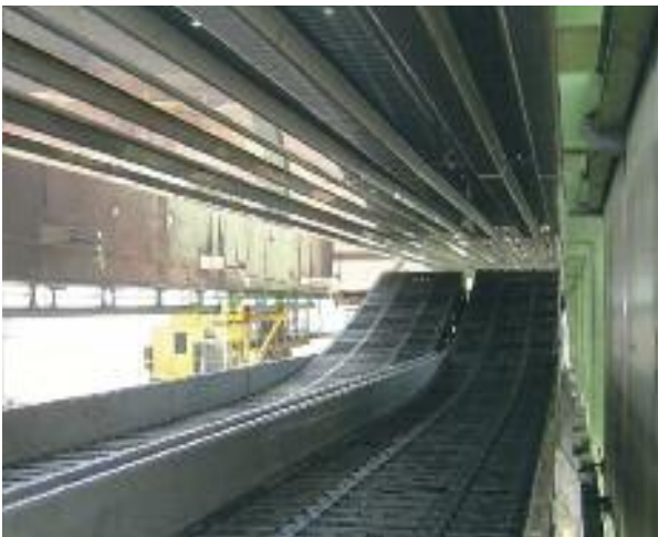
Assembled system in a ship unloading crane with igus® 5050RHD - Travel 248 ft. (106 m), Speed 13.12 ft/s (4 m/s), Fill weight 16.8 lbs/ft (25 kg/m)
