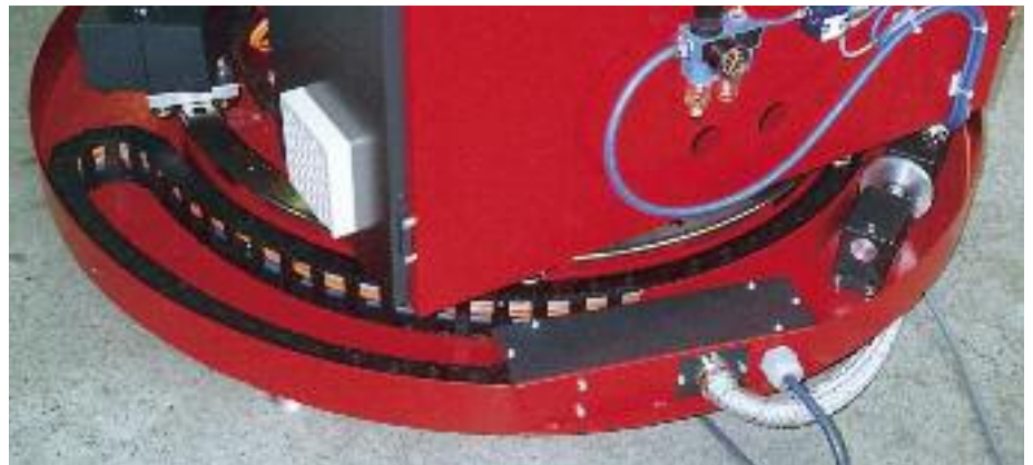
Series 250 with 360° RBR rotary motion on a robot
