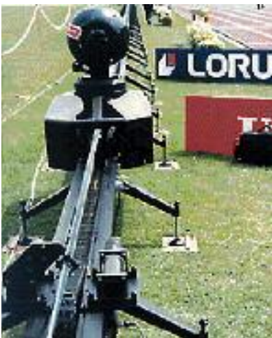
Mobile camera, live images, Olympic Games in Atlanta S = 328 ft (100 m) V = 32.8 ft (10 m/s) in push-pull operation
