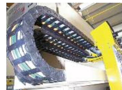
iglus Chainflex® cables permit the smallest bending radius of 5 x d for one million strokes
