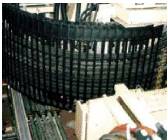
Hydraulics and electric cables are separated from one another in this example
