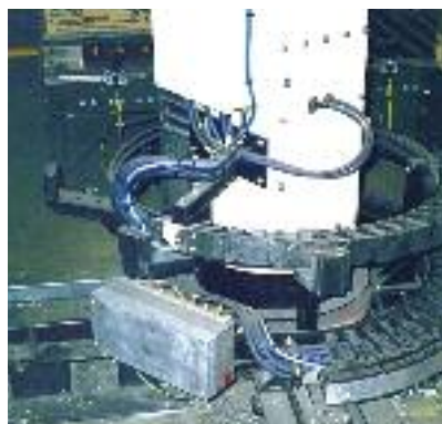
Spiral and rotary movement TwisterChain®
