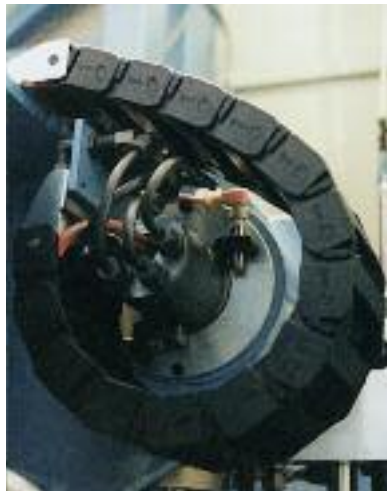
Rotary motion with a "standard" Energy Chain®
