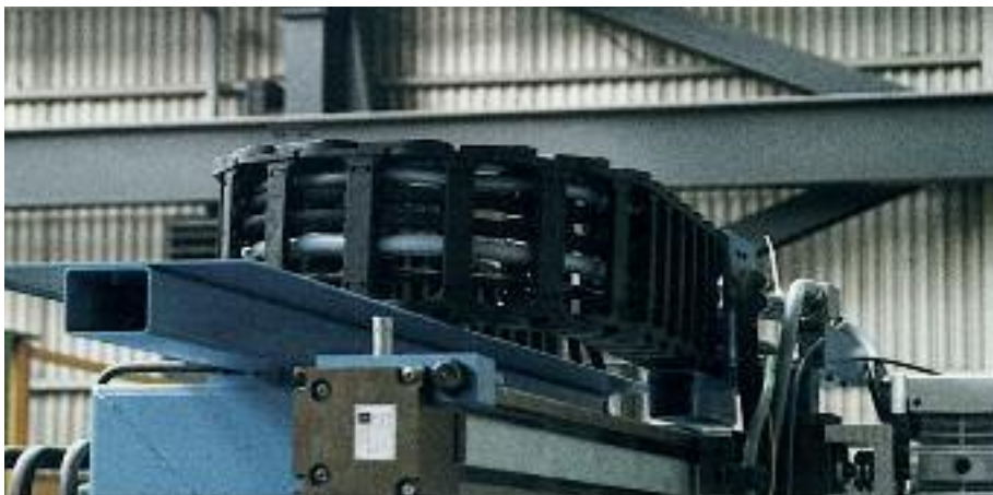
Energy Chain®, side-mounted, supported System E4
