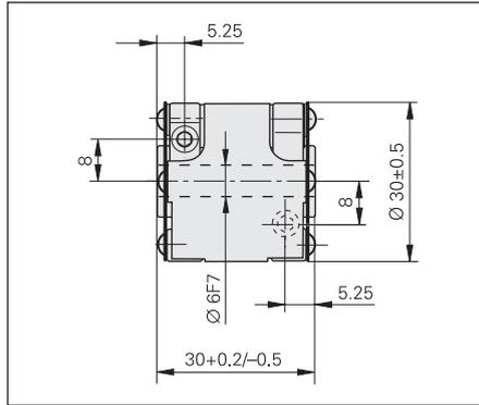
Recommended fit for the customer shaft: h6
