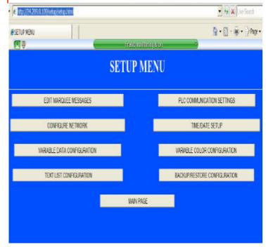
By selecting the "Variable Data Configuration" button, the user can set up the variable data from the plc to be displayed on the marquee sign. The format of the variable data is entered here.
