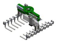
Offers controlled clamping and releasing through the use of pneumatic cylinders, as well as giving the same amount of force on all bags, regardless of bag thickness.
