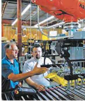
Heavy duty bag gripper shown lifting bags of rock salt off of conveyor during simulated product trials.
