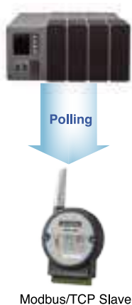
Automation Protocol Modbus/TCP Master
